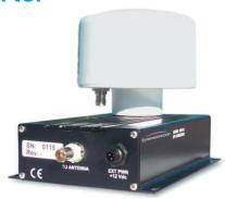
Use the GPS Down/Up converter for cable runs of 250 to 1500 feet (75 m to 457 m). GPS signal down/up conversion is required when signal losses in the antenna cable limit the distance between the receiver and the antenna assembly. The Down/Up Converter may also work with non-Symmetricom L1 GPS receivers. The signal output from the converter is L1 C/A code that can be decoded by any L1 GPS receiver.
