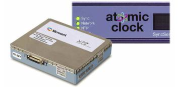
Rubidium atomic clock oscillator upgrades improve holdover accuracy and saves you valuable time. The standard SyncServer is equipped with a temperature compensated crystal oscillator (TCXO) that keeps the server accurate to nanoseconds when tracking GPS. However, if the GPS signal is lost, thereby placing the server in holdover, the TCXO will soon drift away from perfect. Upgrading the oscillator improves the holdover accuracy significantly.
