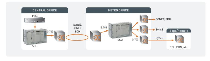
Figure 3: How the existing BITS architecture serves SyncE and legacy
