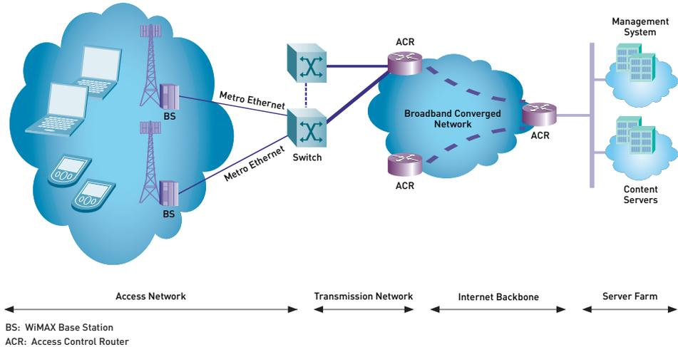
FIG. 1 WiMAX network topology: leveraging core IP network for simplicity & lower capital and operating costs.
