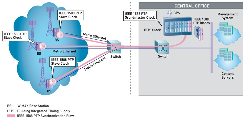
**FIG. 3** Utilizing IEEE 1588 PTP, carriers can reduce the number of GPS-based receivers required in a WiMAX network, significantly reducing deployment cost as well as simplifying network maintenance.
