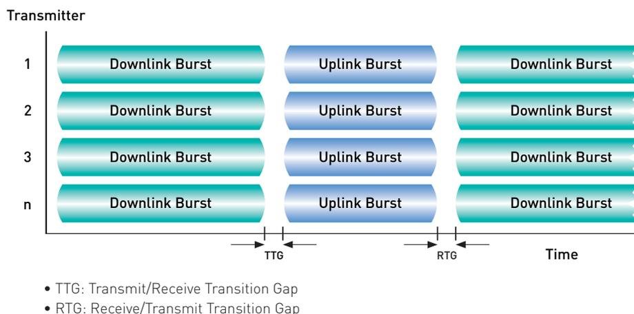
FIG 2 TDD mode requires tight time synchronization to prevent interference.
