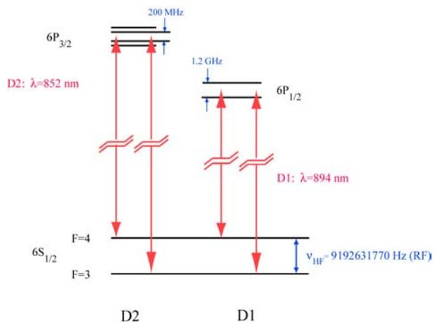
**Figure 6:** Cesium D1 and D2 CPT resonance levels
