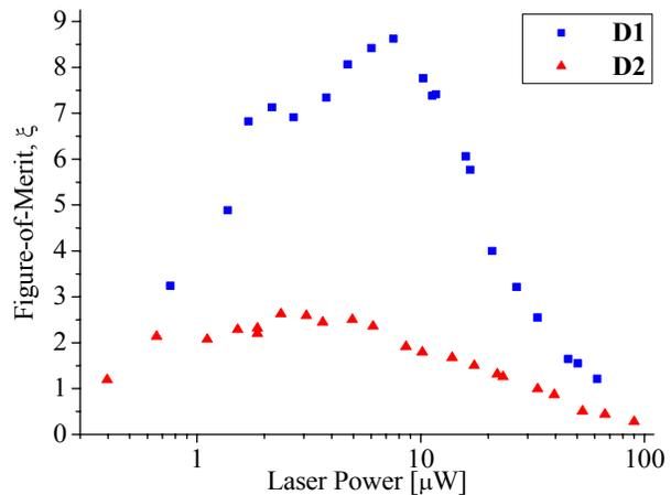
**Figure 10:** D1 vs. D2 figure-of-merit vs. laser power
