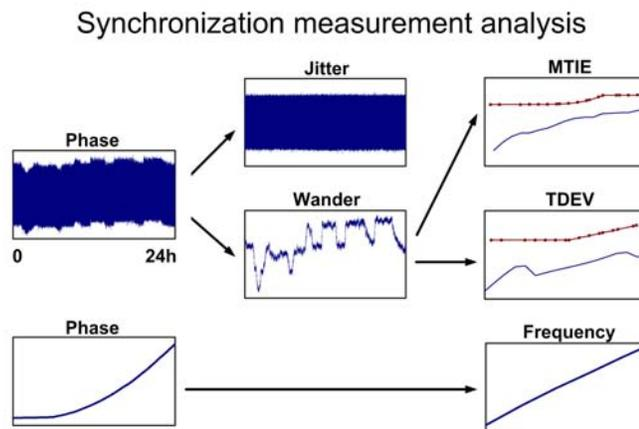
**Fig. 2.** Measurements used by Telcordia, ANSI, ETSI and ITU-T to characterize synchronization (phase, frequency, MTIE and TDEV) are all derived from phase. A high-pass filter applied to phase reveals jitter while a low-pass filter applied to phase reveals wander.
