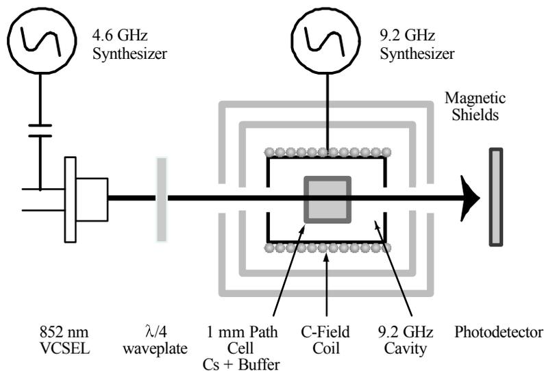
**Figure 4: Schematic of dual-mode CSAC testbed**
