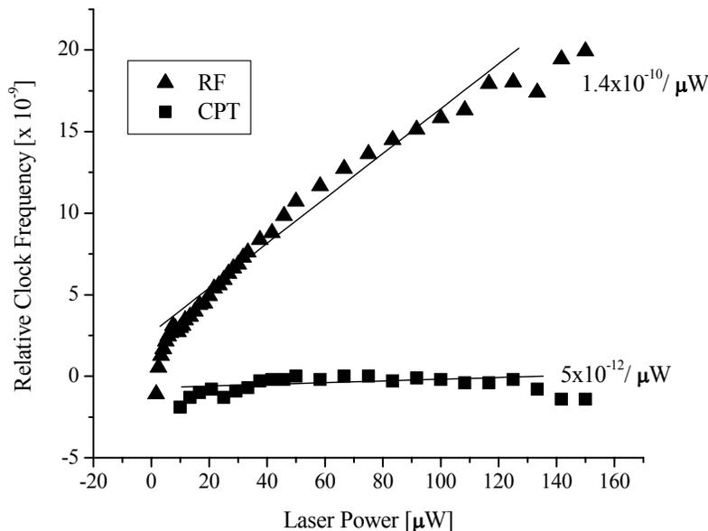
**Figure 11: Light shift of RF and CPT interrogation**
