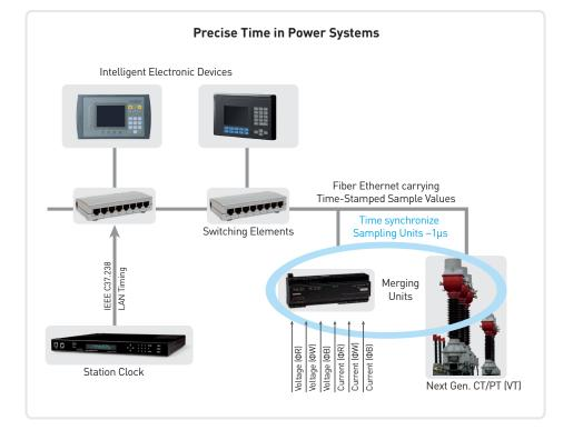
Figure 1: Devices in a Power Substation
