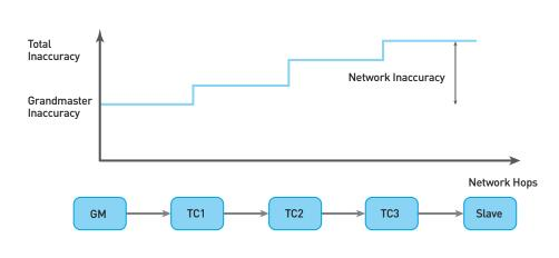
Figure 5: Inaccuracy Accumulation in a Power Profile Network
