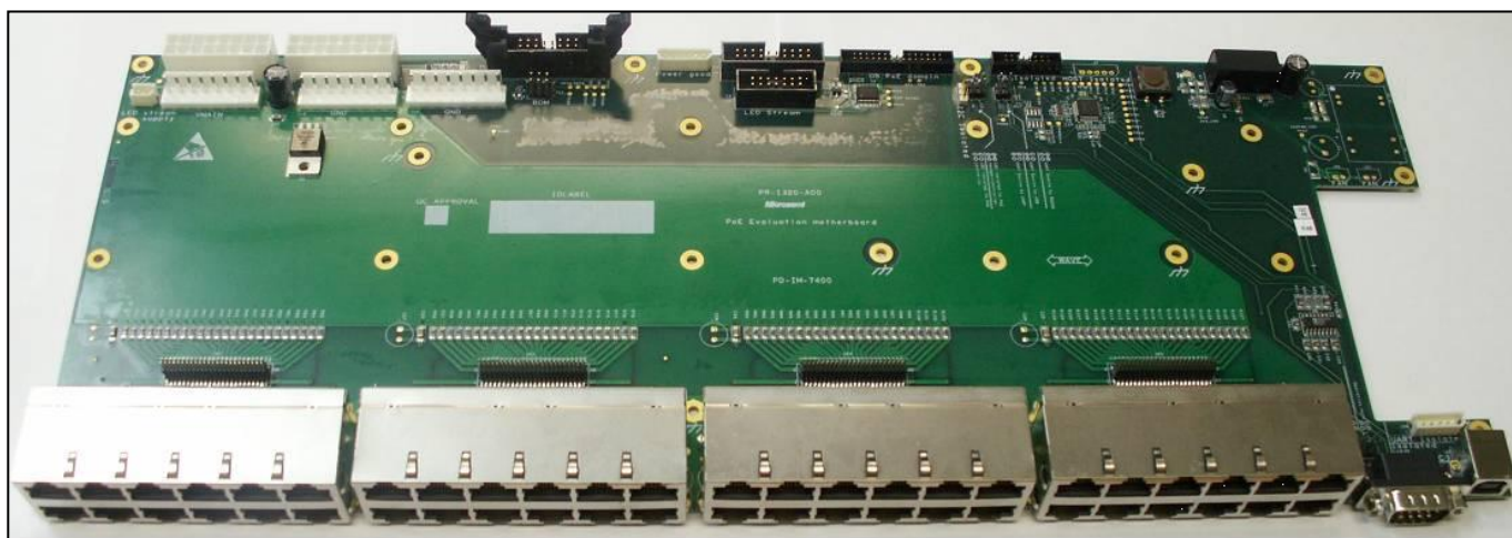
Figure 2: PD-IM-7500 MB (Motherboard) Evaluation Board – General View
