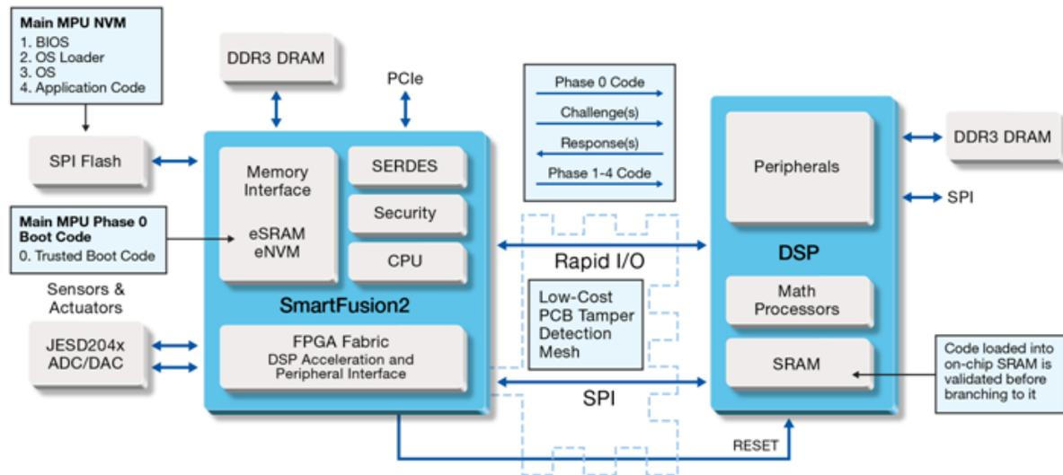
Figure 4: Secure Embedded Industrial Sensor Controller
