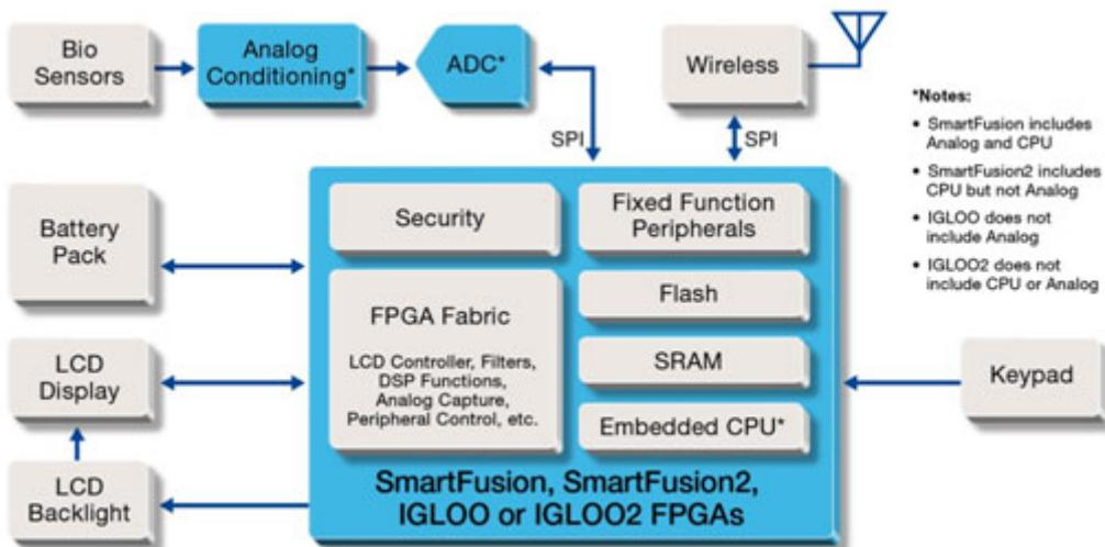
Figure 2: Block Diagram of the Design for a Personal Health Monitor
