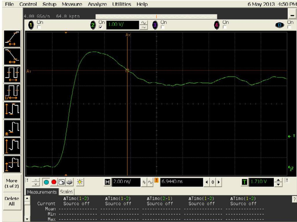
Figure 13a DUT 577 Pre-Irradiation Rising Edge
