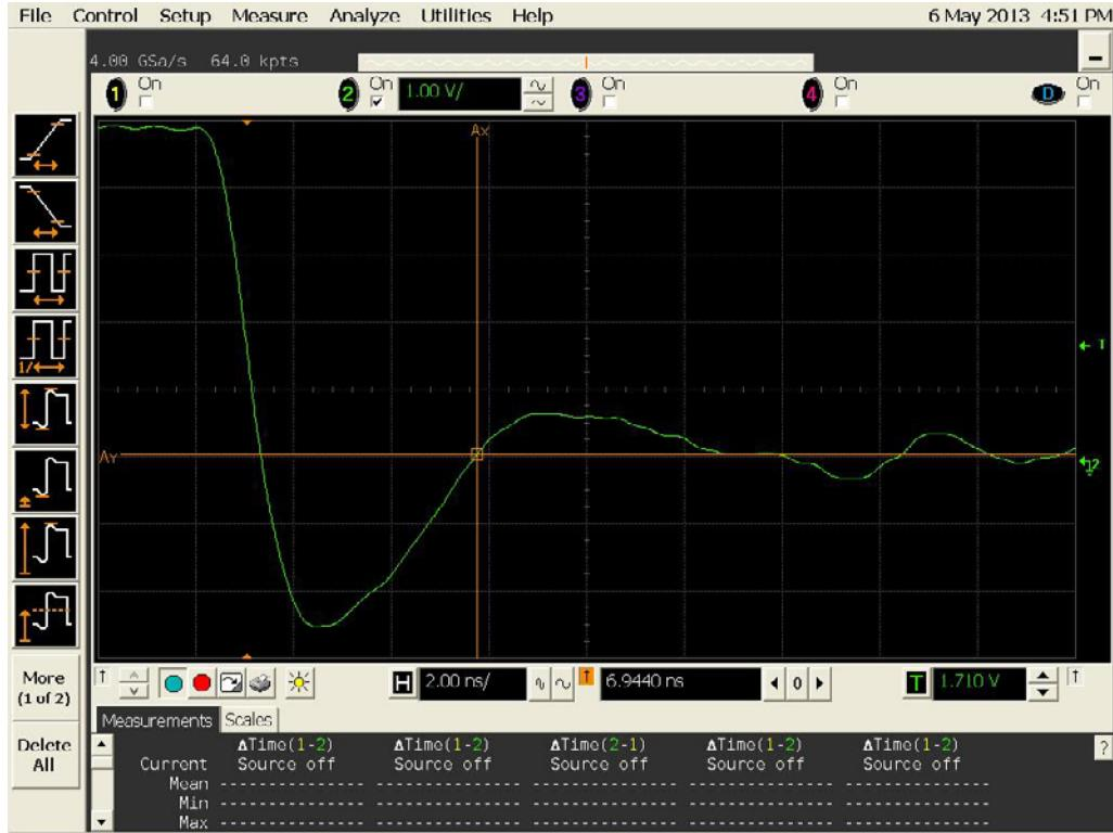
Figure 19a DUT 577 Pre-Irradiation Falling Edge
