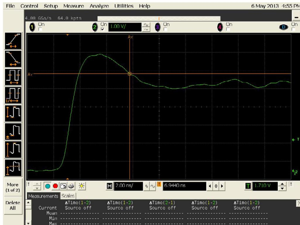
Figure 14a DUT 583 Pre-Irradiation Rising Edge
