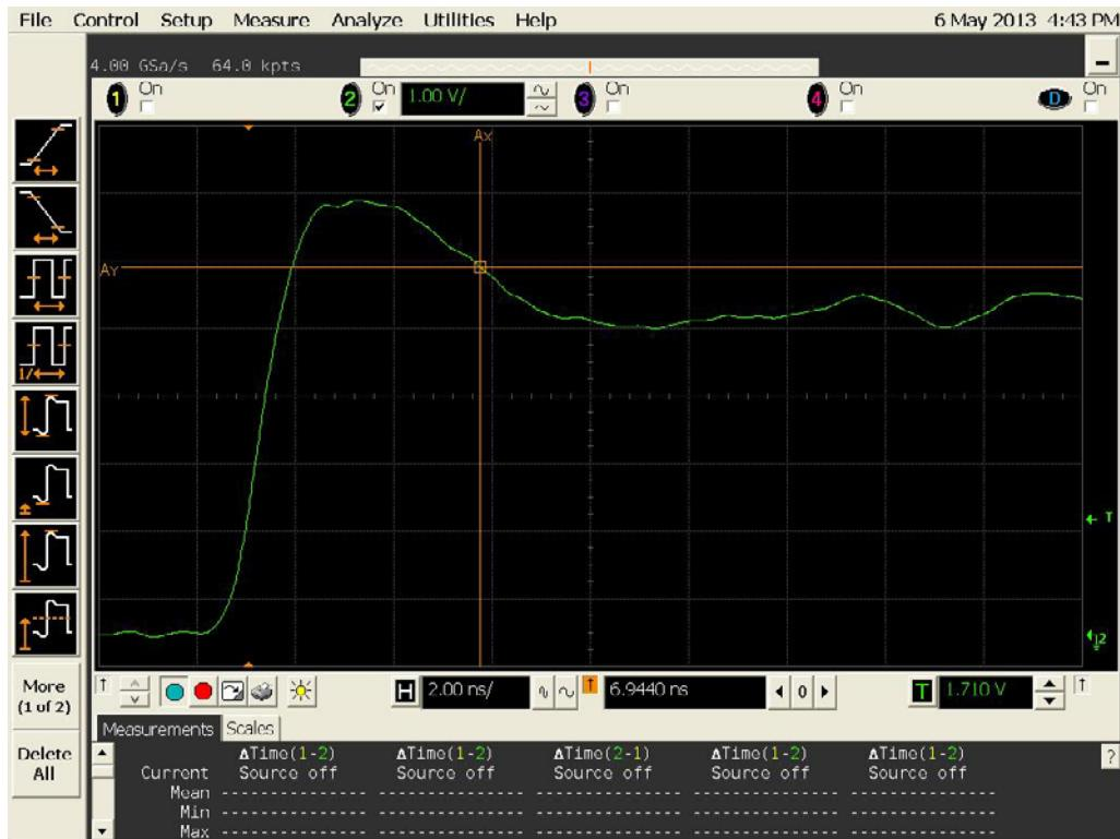
Figure 11a DUT 536 Pre-Radiation Rising Edge
