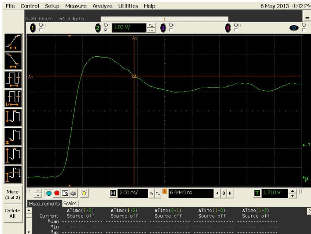
Figure 10a DUT 518 Pre-Irradiation Rising Edge
