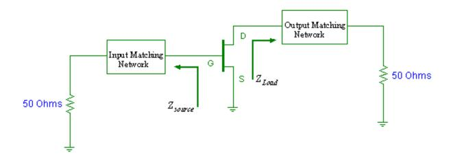
Note:  $Z_{in}$  is looking into the input circuit;  $Z_{Load}$  is looking into the output circuit.
