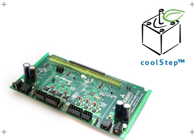
**INFO** The TRINAMIC TCMC-AC-840 Daughter Board Kit is an FPGA prototyping platform for power drivers for brushless DC motors (BLDC) as well as stepper motors. The TCMC-AC-840 Daughter Board Kit incorporates one TMC603A BLDC motor driver IC and one TMC262 coolStep™ stepper motor driver IC as well as two fitting motors to start prototyping right away.
