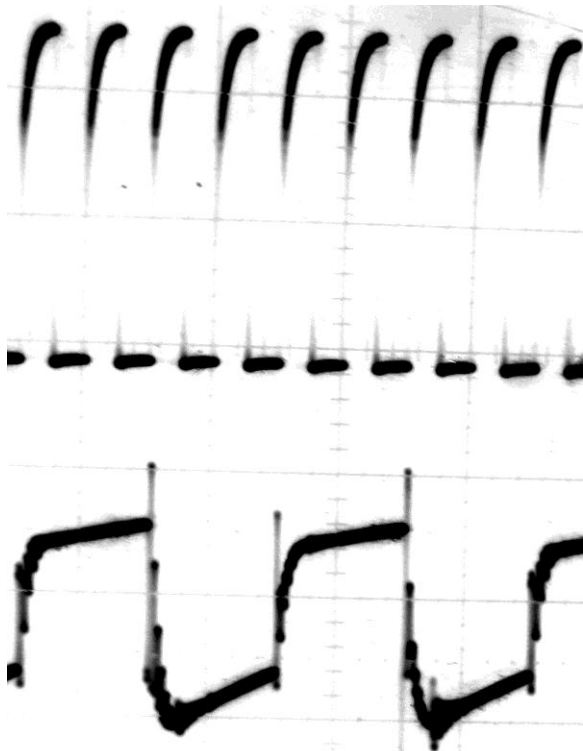
Figure 6: Solder Joint BIST – Input Clock (top) and Signal Across the Capacitor (bottom): 2\mu\text{s} \times 2.0\text{V} Grid.
