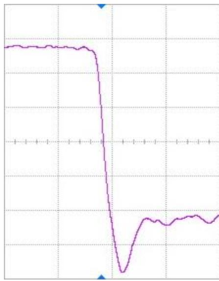
Figure 10(a) DUT 1848 pre-irradiation falling edge, abscissa scale is 1 V/div and ordinate scale is 5 ns/div.
