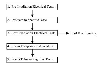
Figure 1. Test Method Flow Chart
