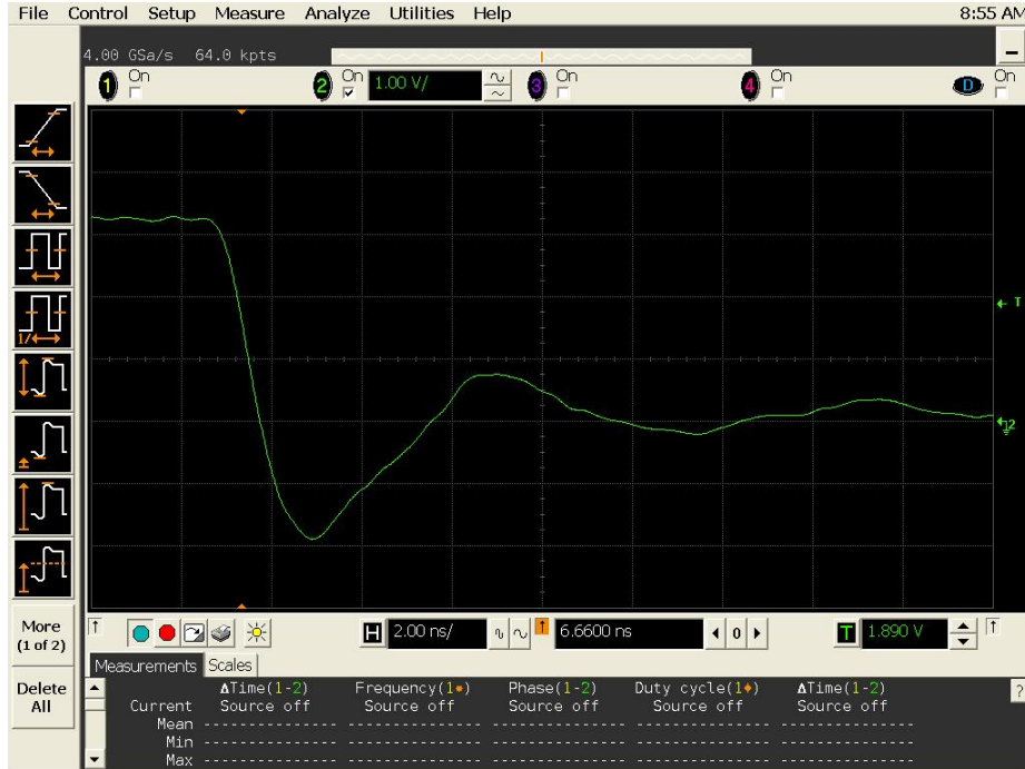
Figure 19a DUT 18281 Pre-Irradiation Falling Edge, abscissa scale is 1 V/div and ordinate scale is 2 ns/div.
