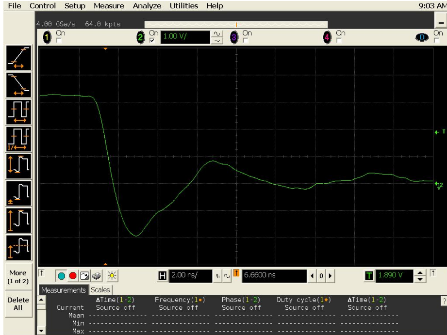
Figure 17a DUT 18273 Pre-Irradiation Falling Edge, abscissa scale is 1 V/div and ordinate scale is 2 ns/div.
