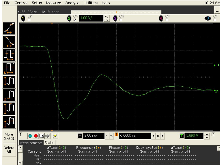
Figure 19a DUT 18086 Pre-Irradiation Falling Edge, abscissa scale is 1 V/div and ordinate scale is 2 ns/div.
