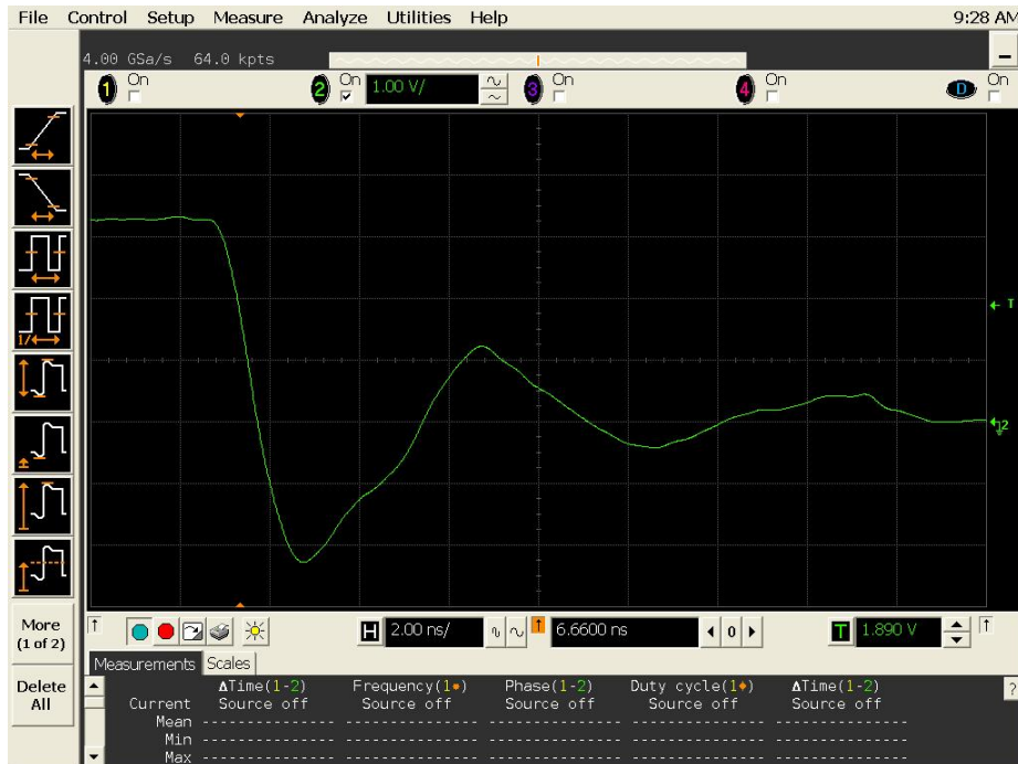
Figure 15b DUT 18063 Post-Annealing Falling Edge, abscissa scale is 1 V/div and ordinate scale is 2 ns/div.
