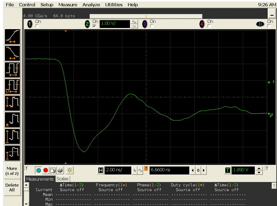
Figure 14b DUT 18061 Post-Annealing Falling Edge, abscissa scale is 1 V/div and ordinate scale is 2 ns/div.
