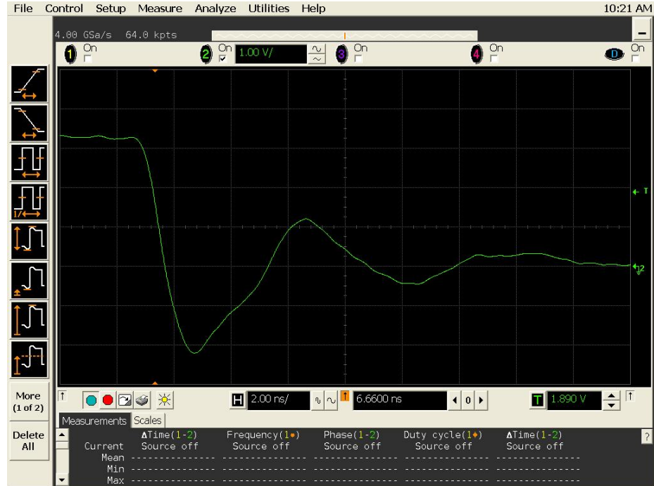
Figure 14a DUT 18061 Pre-Irradiation Falling Edge, abscissa scale is 1 V/div and ordinate scale is 2 ns/div.
