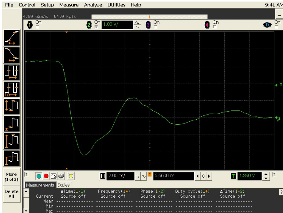
Figure 19b DUT 18086 Post-Annealing Falling Edge, abscissa scale is 1 V/div and ordinate scale is 2 ns/div.
