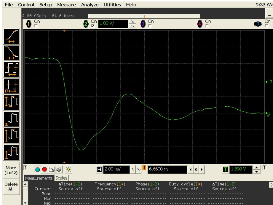
Figure 17b DUT 18076 Post-Annealing Falling Edge, abscissa scale is 1 V/div and ordinate scale is 2 ns/div.
