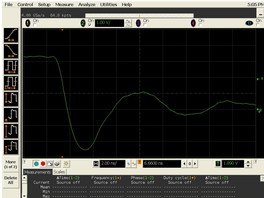
Figure 17b DUT 14943 Post-Annealing Falling Edge, abscissa scale is 1 V/div and ordinate scale is 2 ns/div.
