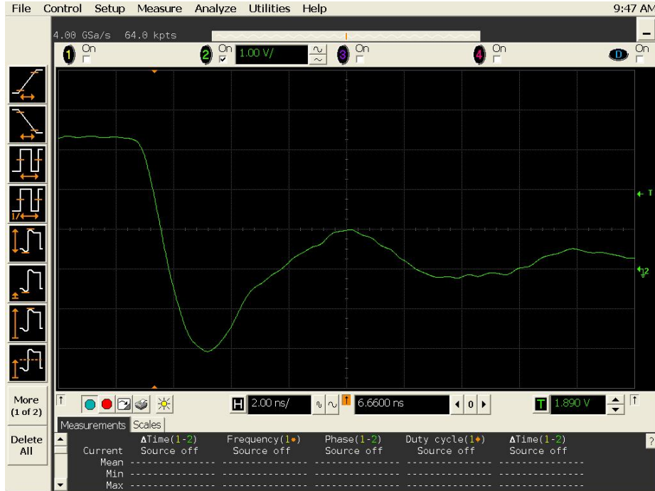
Figure 17a DUT 14943 Pre-Irradiation Falling Edge, abscissa scale is 1 V/div and ordinate scale is 2 ns/div.
