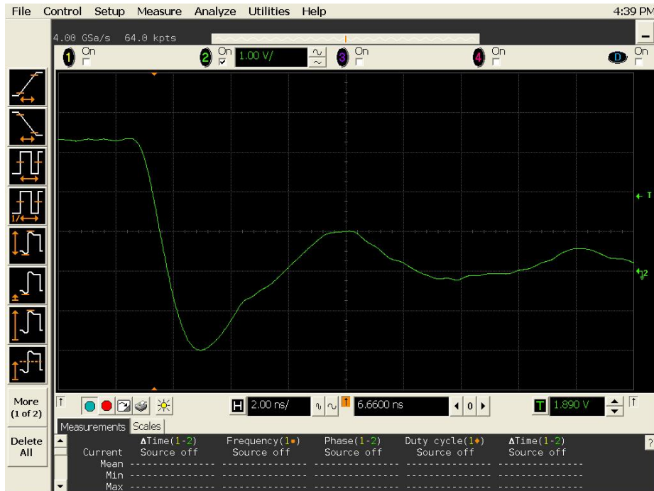
Figure 19b DUT 14955 Post-Annealing Falling Edge, abscissa scale is 1 V/div and ordinate scale is 2 ns/div.
