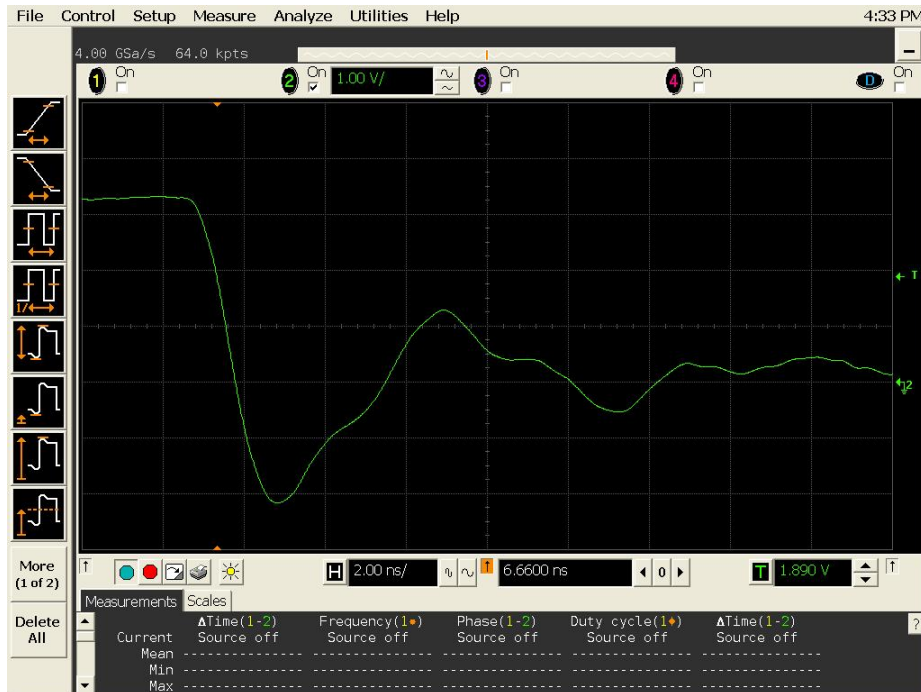
Figure 19b DUT 10971 Post-Annealing Falling Edge, abscissa scale is 1 V/div and ordinate scale is 2 ns/div.
