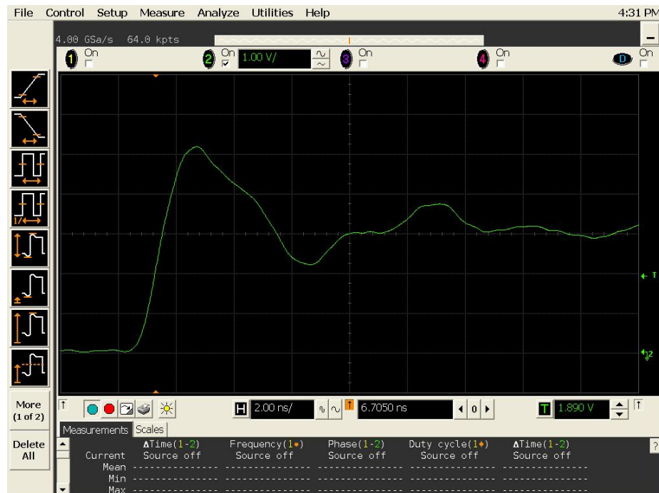
Figure 12b DUT 10970 Post-Annealing Rising Edge, abscissa scale is 1 V/div and ordinate scale is 2 ns/div.
