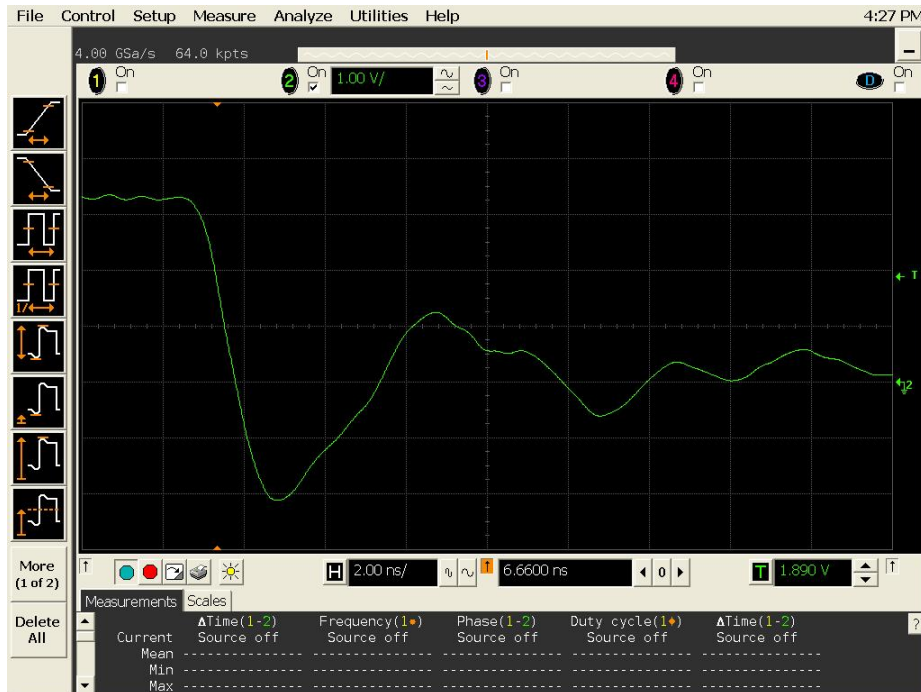
Figure 17b DUT 10964 Post-Annealing Falling Edge, abscissa scale is 1 V/div and ordinate scale is 2 ns/div.
