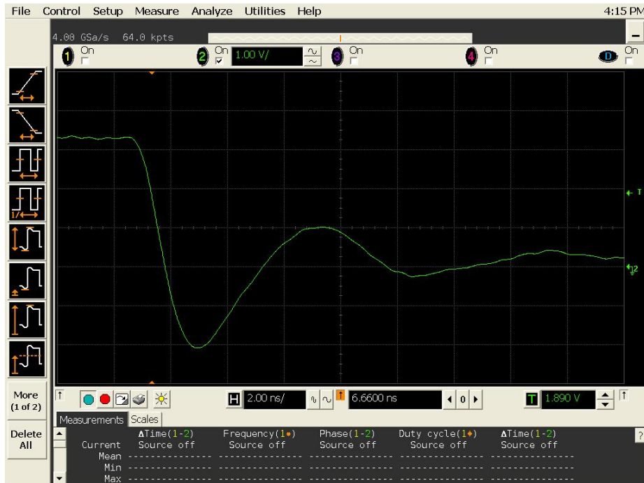
Figure 15b DUT 10958 Post-Annealing Falling Edge, abscissa scale is 1 V/div and ordinate scale is 2 ns/div.
