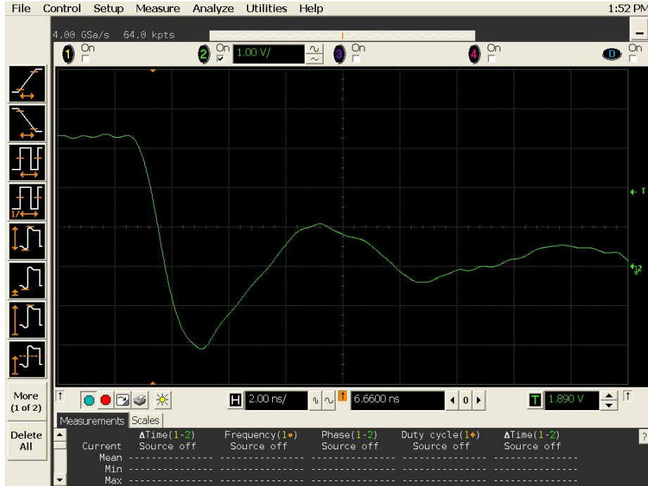
Figure 19a DUT 10971 Pre-Irradiation Falling Edge, abscissa scale is 1 V/div and ordinate scale is 2 ns/div.
