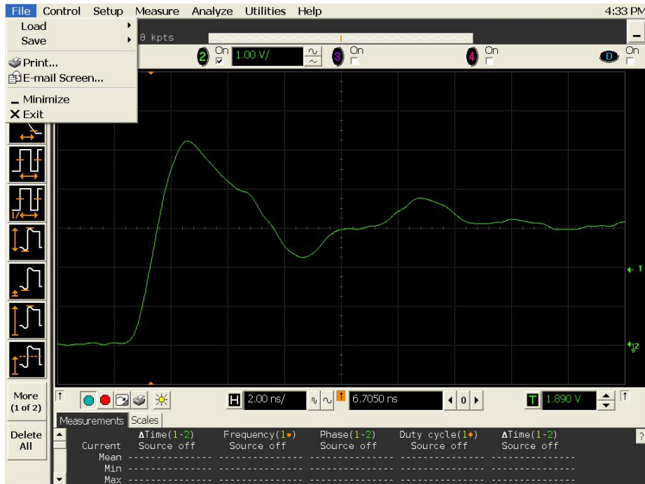
Figure 13b DUT 10971 Post-Annealing Rising Edge, abscissa scale is 1 V/div and ordinate scale is 2 ns/div.
