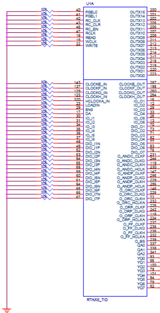
Figure A1 I/O Bias During Irradiation
