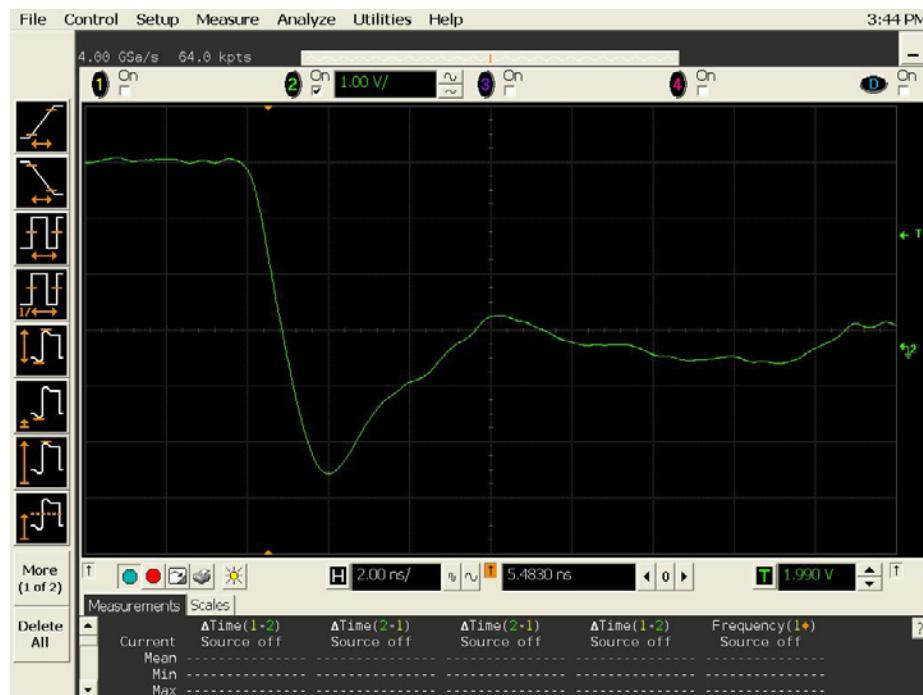
**Figure 15a DUT 8236 Pre-Irradiation Falling Edge, abscissa scale is 1 V/div and ordinate scale is 2 ns/div.**
