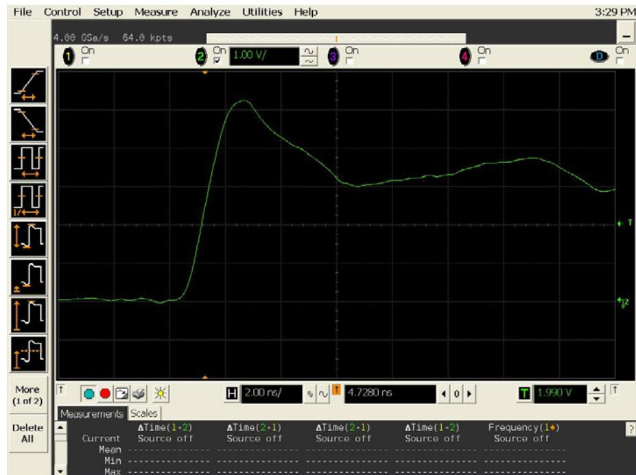
**Figure 9a** DUT 8231 Pre-Irradiation Rising Edge,
