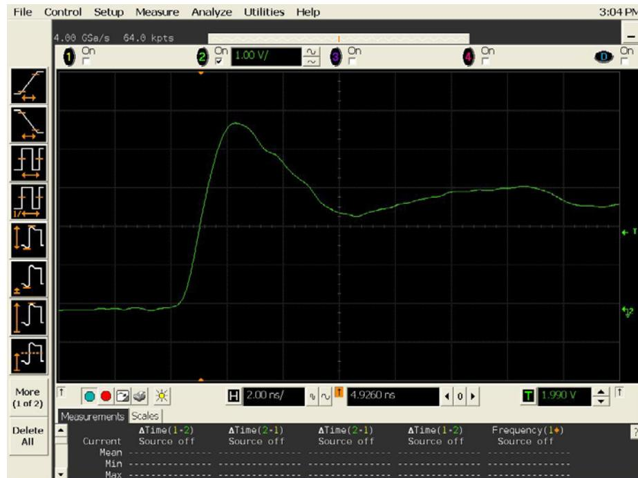
**Figure 7b DUT 8196 Post-Annealing Rising Edge,
