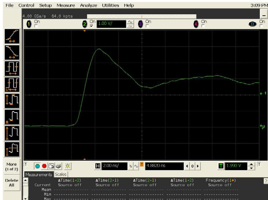
**Figure 9b** DUT 8231 Post-Annealing Rising Edge,
