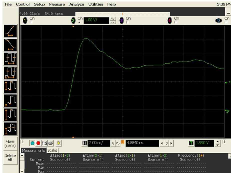
**Figure 7a DUT 8196 Pre-Irradiation Rising Edge,
