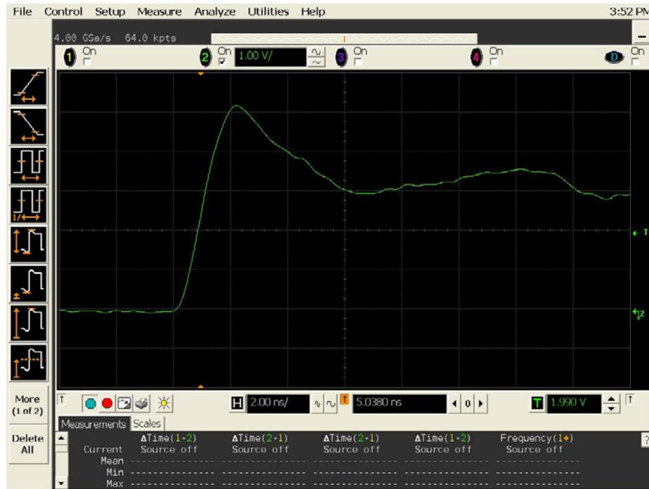
**Figure 8a DUT 8198 Pre-irradiation Rising Edge,
