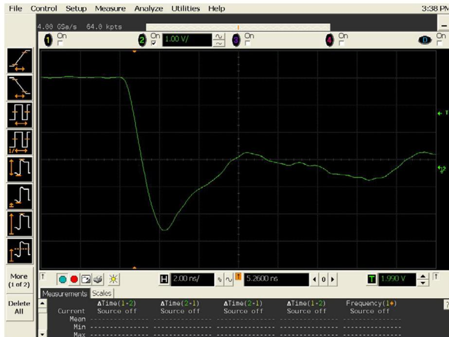
Figure 12a DUT 8196 Pre-Irradiation Falling Edge,
