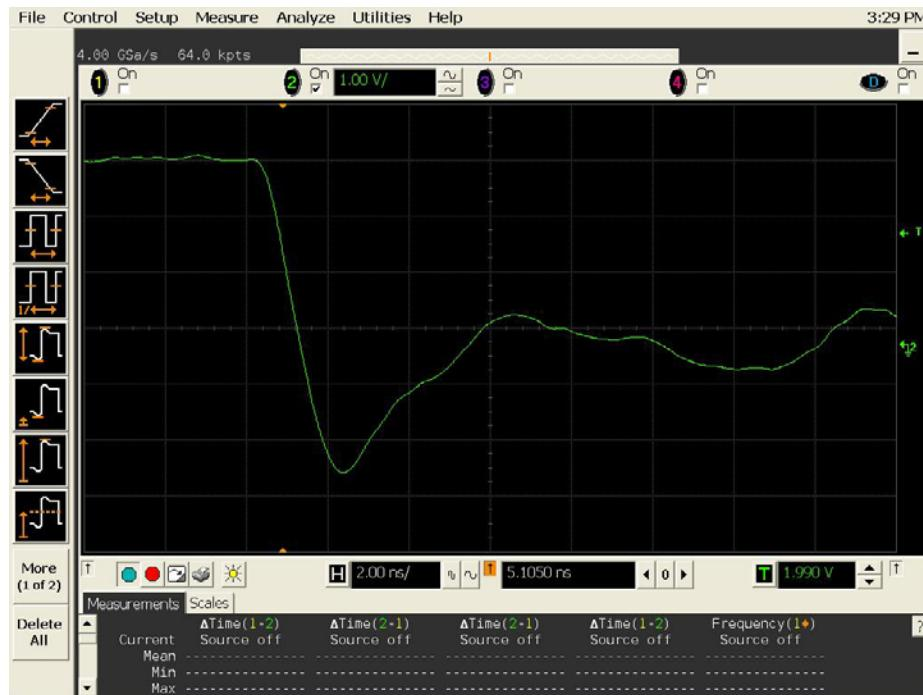
Figure 14a DUT 8231 Pre-Irradiation Falling Edge,
