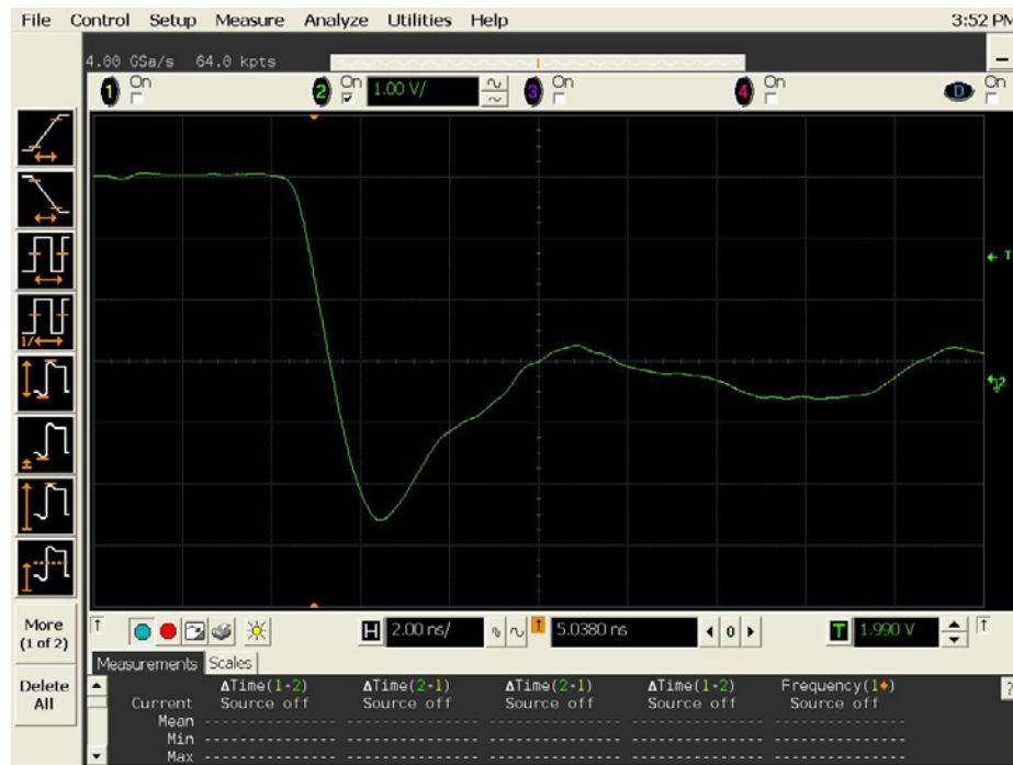
**Figure 13a DUT 8198 Pre-Irradiation Falling Edge,
