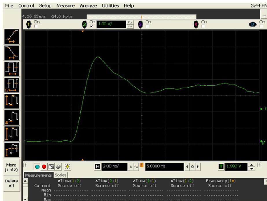
Figure 10a DUT 8236 Pre-Irradiation Rising Edge,
