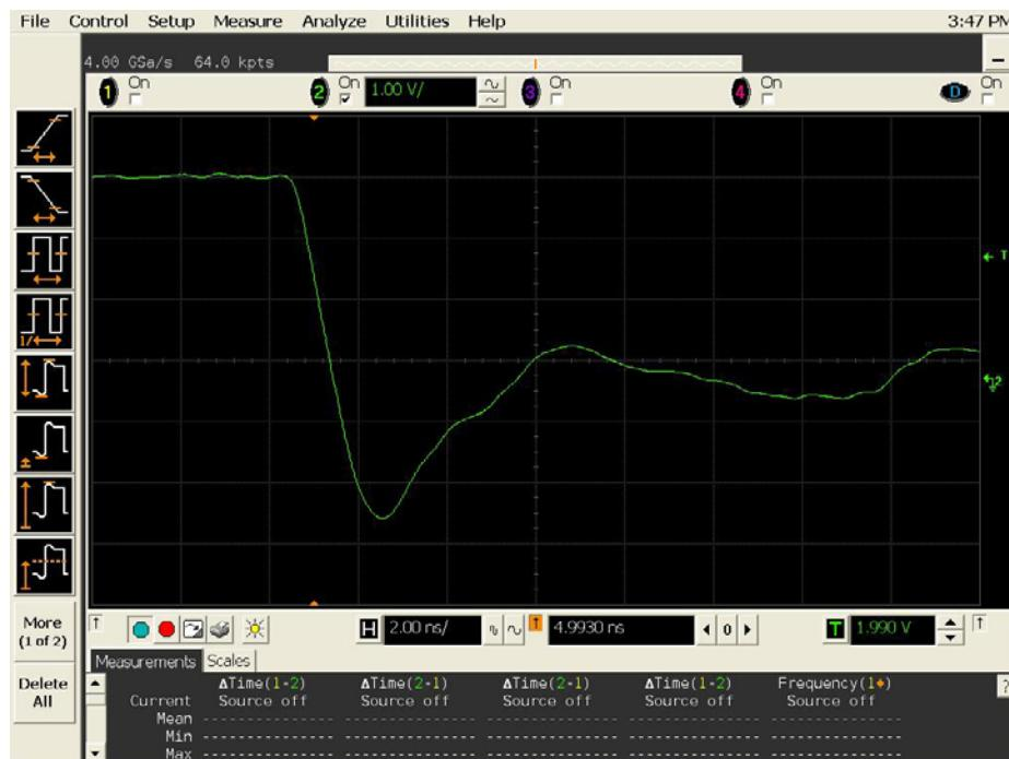
Figure 16a DUT 8237 Pre-Irradiation Falling Edge,
