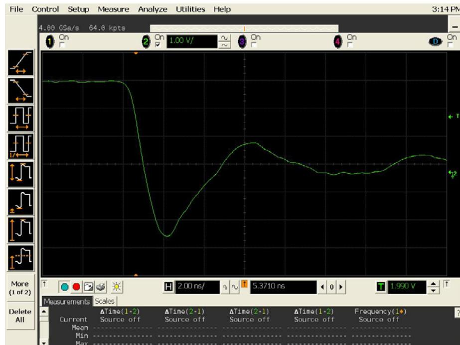
**Figure 13b DUT 8198 Post-Annealing Falling Edge,
