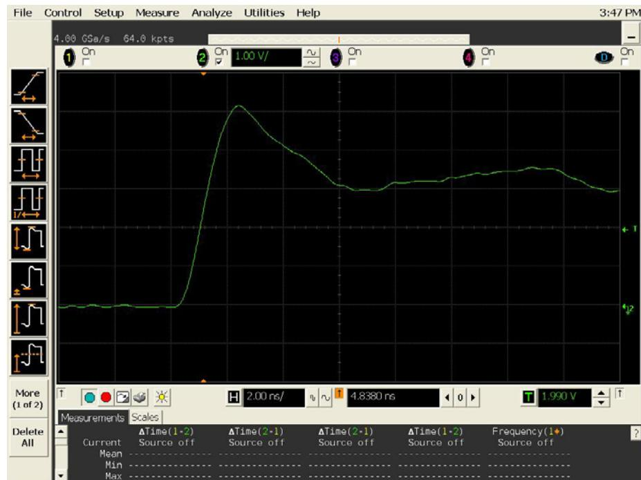
**Figure 11a** DUT 8237 Pre-Irradiation Rising Edge,
