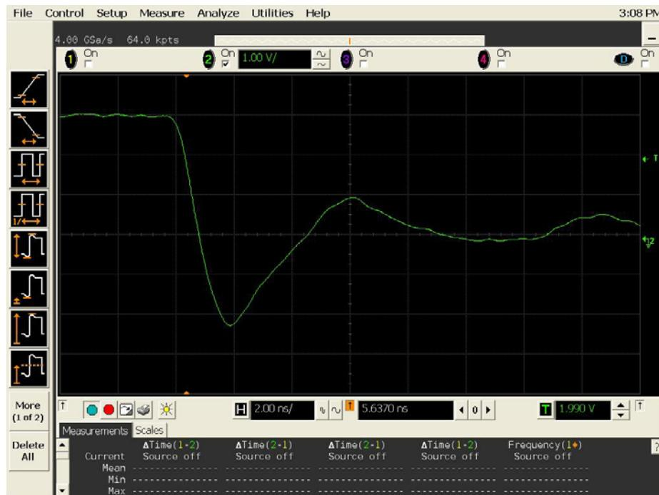
Figure 14b DUT 8231 Post-Annealing Falling Edge,
