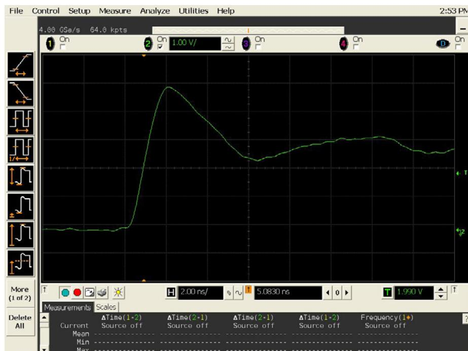
Figure 10b DUT 8236 Post-Annealing Rising Edge,
