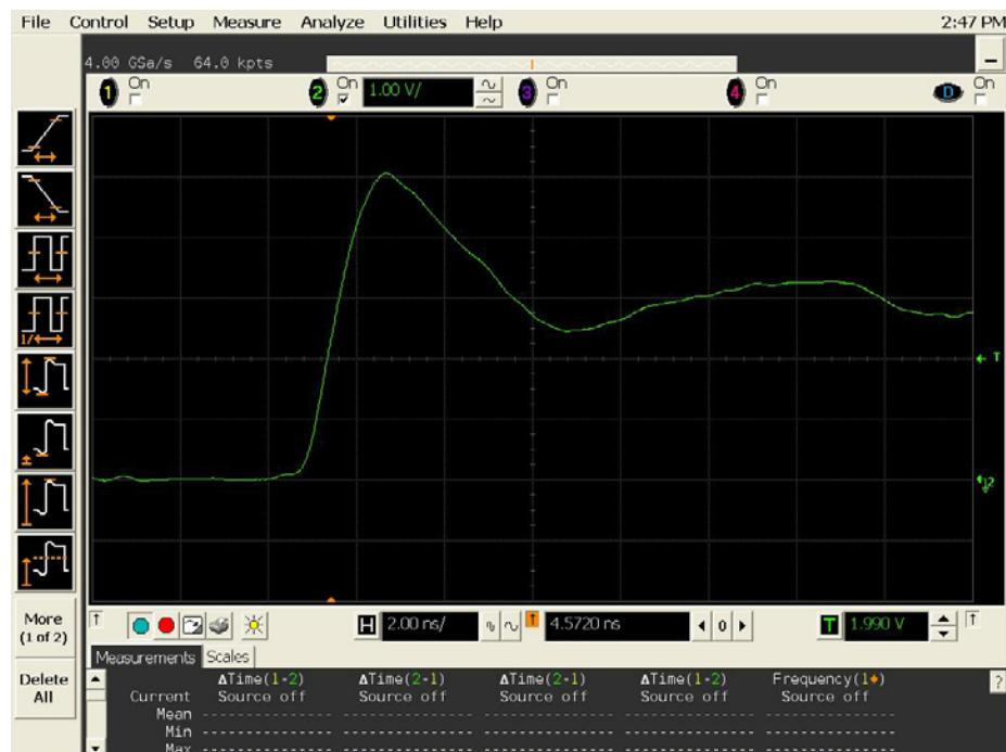
**Figure 11b** DUT 8237 Post-Annealing Rising Edge,
