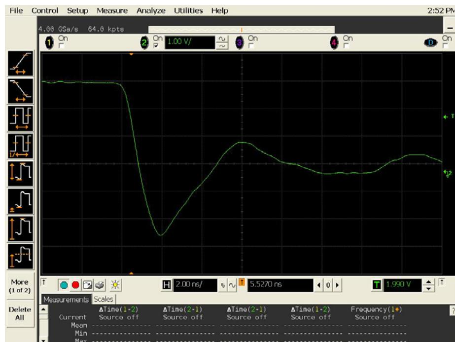
Figure 15b DUT 8236 Post-Annealing Falling Edge, abscissa scale is 1 V/div and ordinate scale is 2 ns/div.
