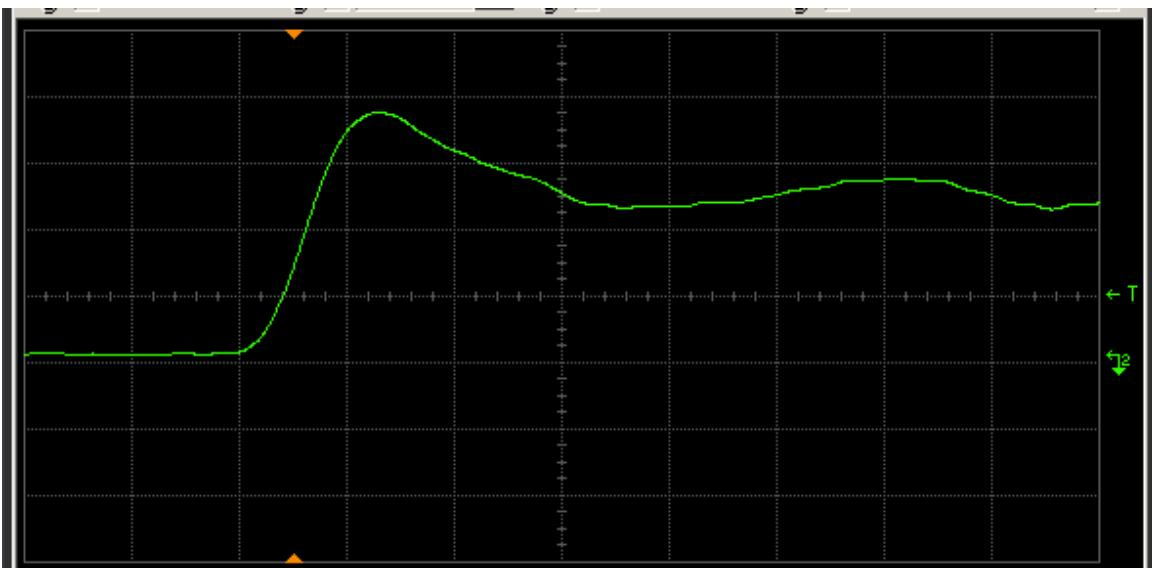
Figure 12(b) DUT 225 post-annealing rising edge. The ordinate is 2 V/div, and abscissa 2 ns/div.
