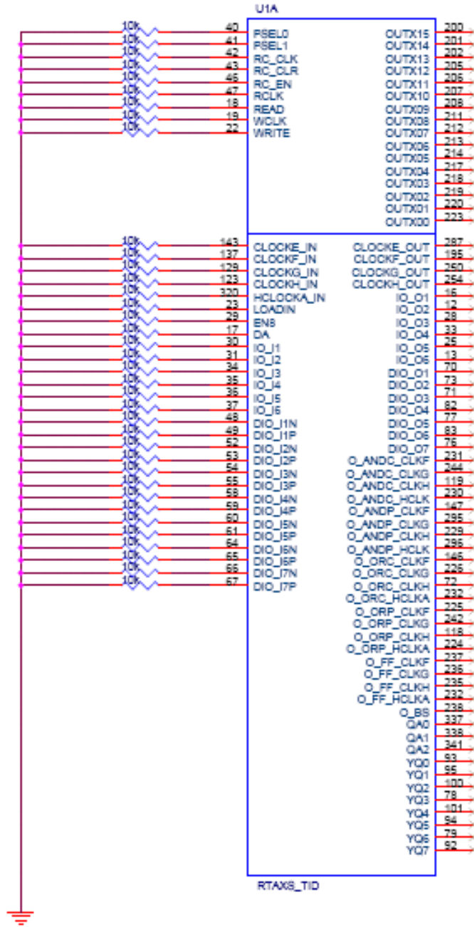
Figure A1 IO bias during irradiation
