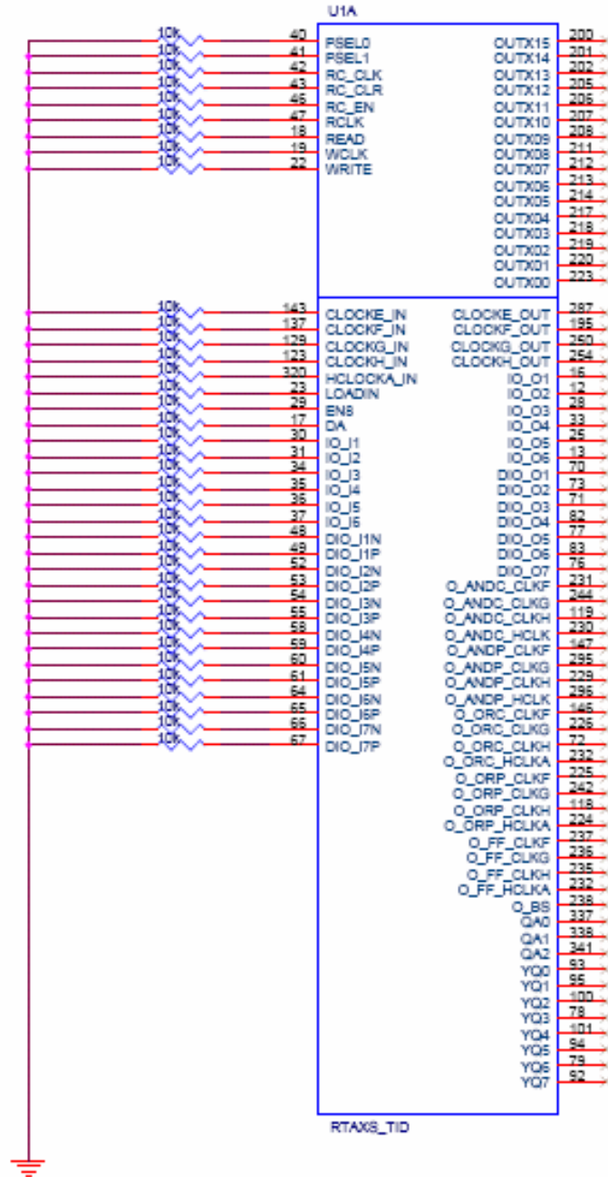
Figure A1 IO bias during irradiation
