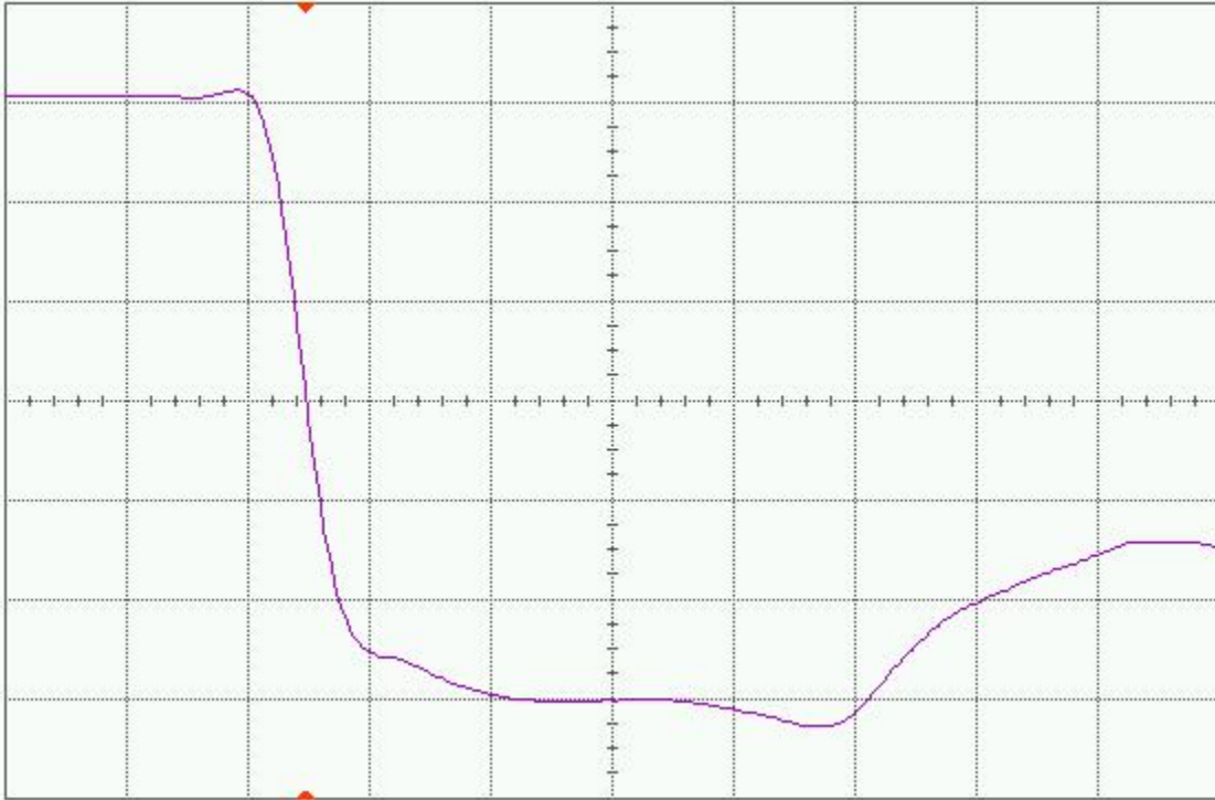
Figure 16(b) DUT3 post-annealing falling edge, abscissa scale is 1 V/div and ordinate scale is 2 ns/div.
