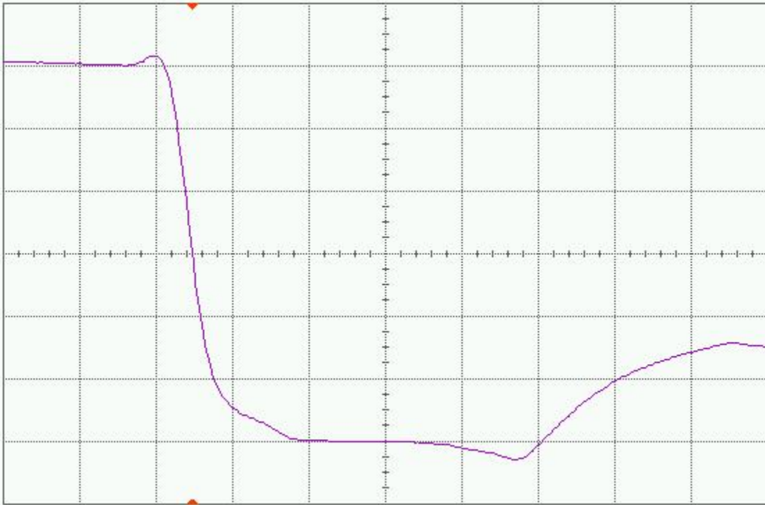
Figure 15(b) DUT2 post-annealing falling edge, abscissa scale is 1 V/div and ordinate scale is 2 ns/div.
