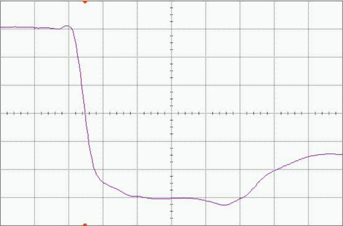
Figure 17(b) DUT4 post-annealing falling edge, abscissa scale is 1 V/div and ordinate scale is 2 ns/div.
