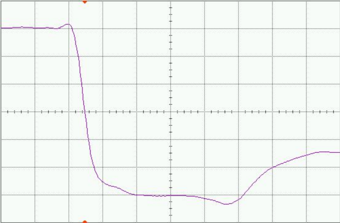
Figure 18(b) DUT5 post-annealing falling edge, abscissa scale is 1 V/div and ordinate scale is 2 ns/div.
