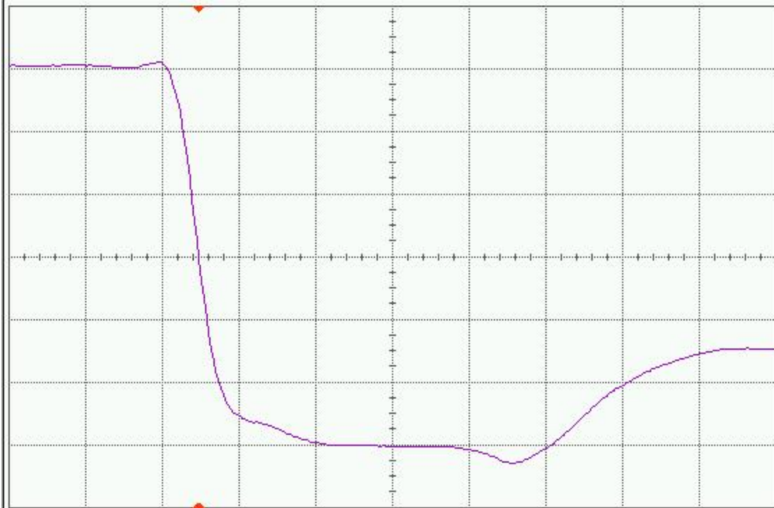
Figure 14(b) DUT1 post-annealing falling edge, abscissa scale is 1 V/div and ordinate scale is 2 ns/div.
