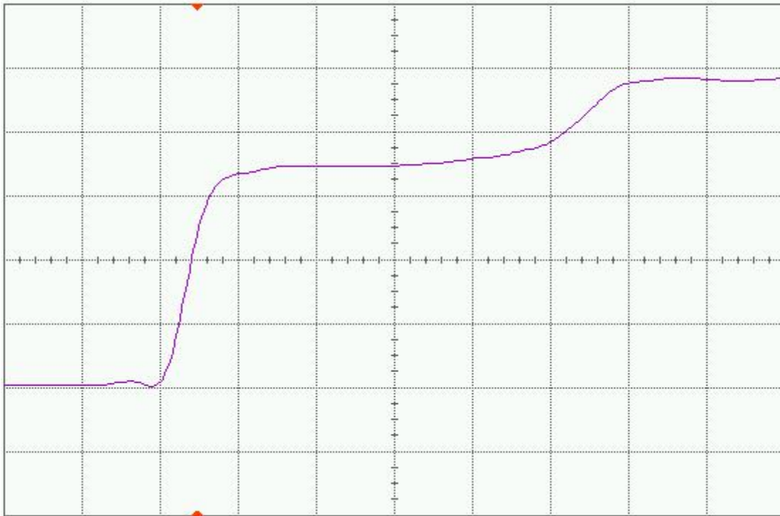
Figure 9(b) DUT1 post-annealing rising edge, abscissa scale is 1 V/div and ordinate scale is 2 ns/div.
