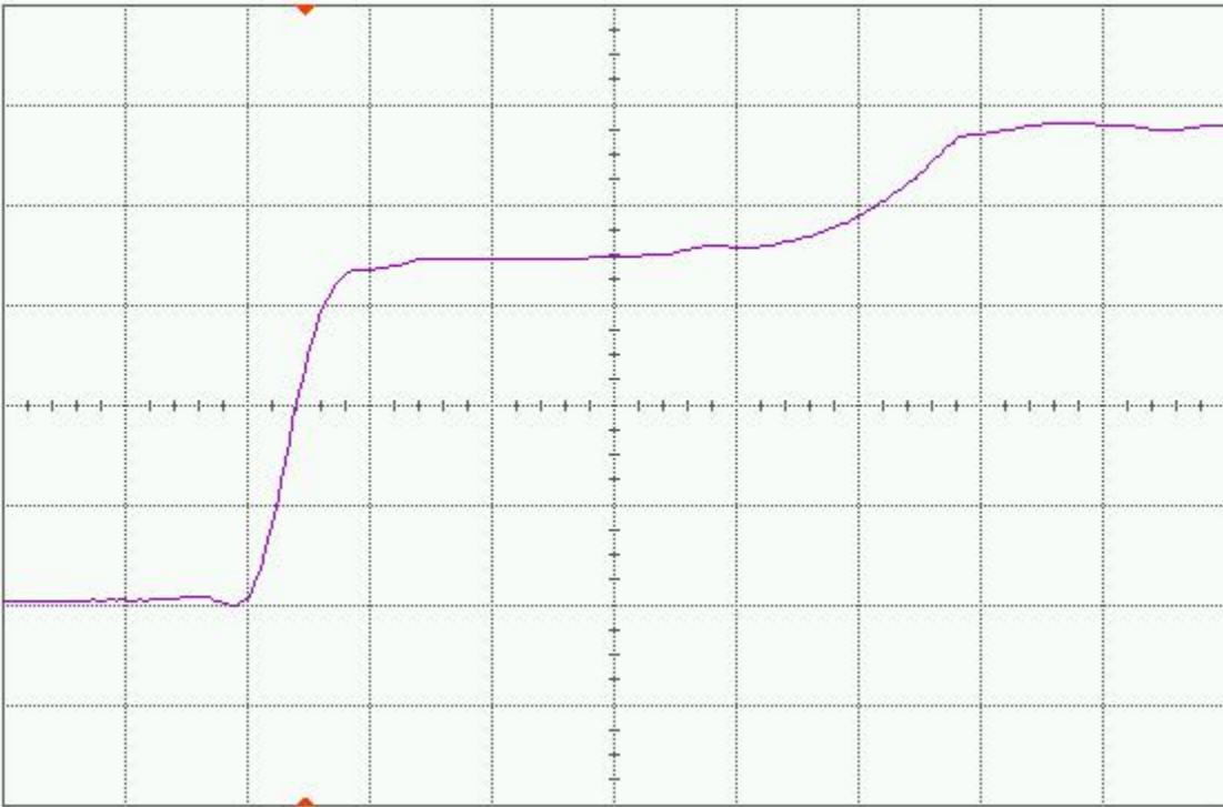
Figure 12(b) DUT4 post-annealing rising edge, abscissa scale is 1 V/div and ordinate scale is 2 ns/div.
