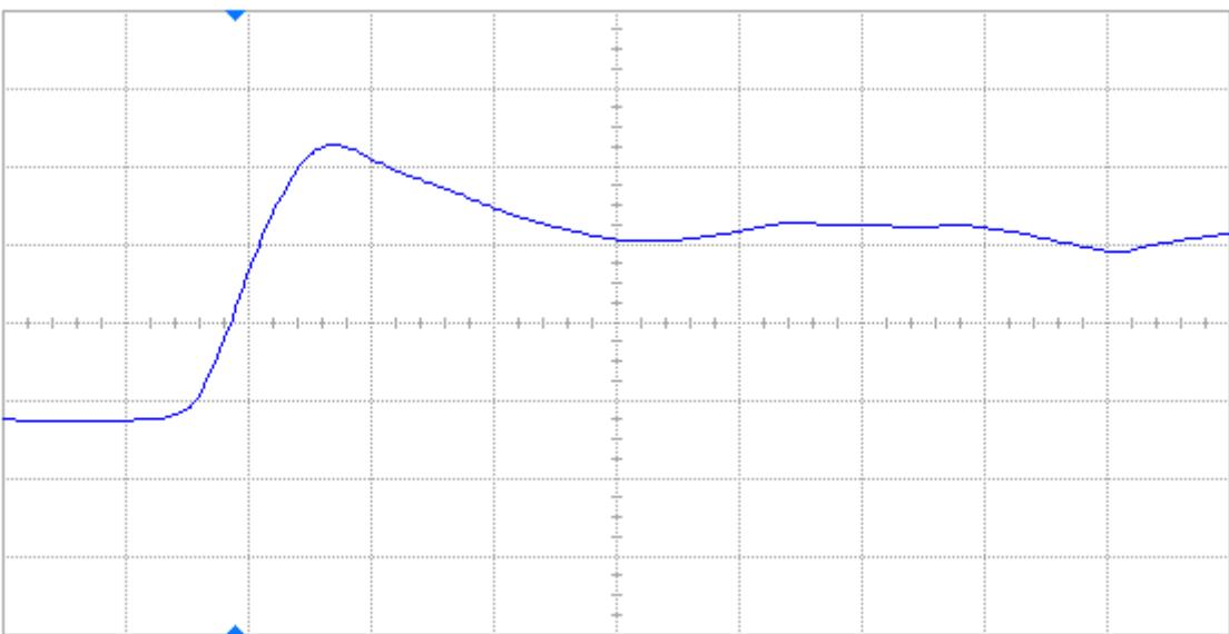
Figure 16 Post-annealing rising edge of DUT 67774, abscissa scale is 2 V/div and ordinate scale is 2 ns/div.
