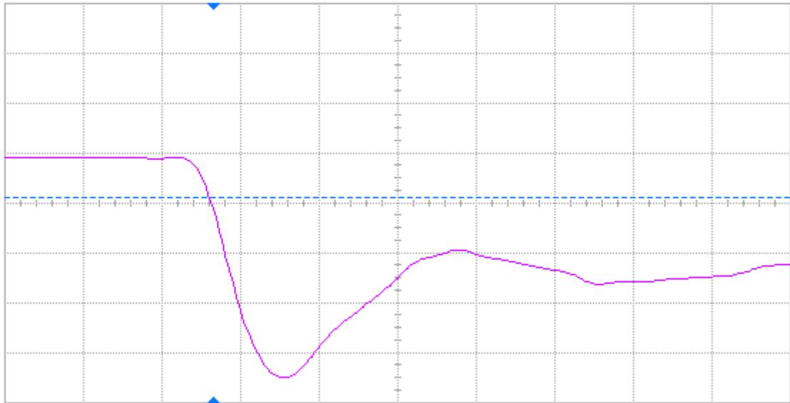
Figure 25 Pre-annealing falling edge of DUT 67774, abscissa scale is 2 V/div and ordinate scale is 2 ns/div.
