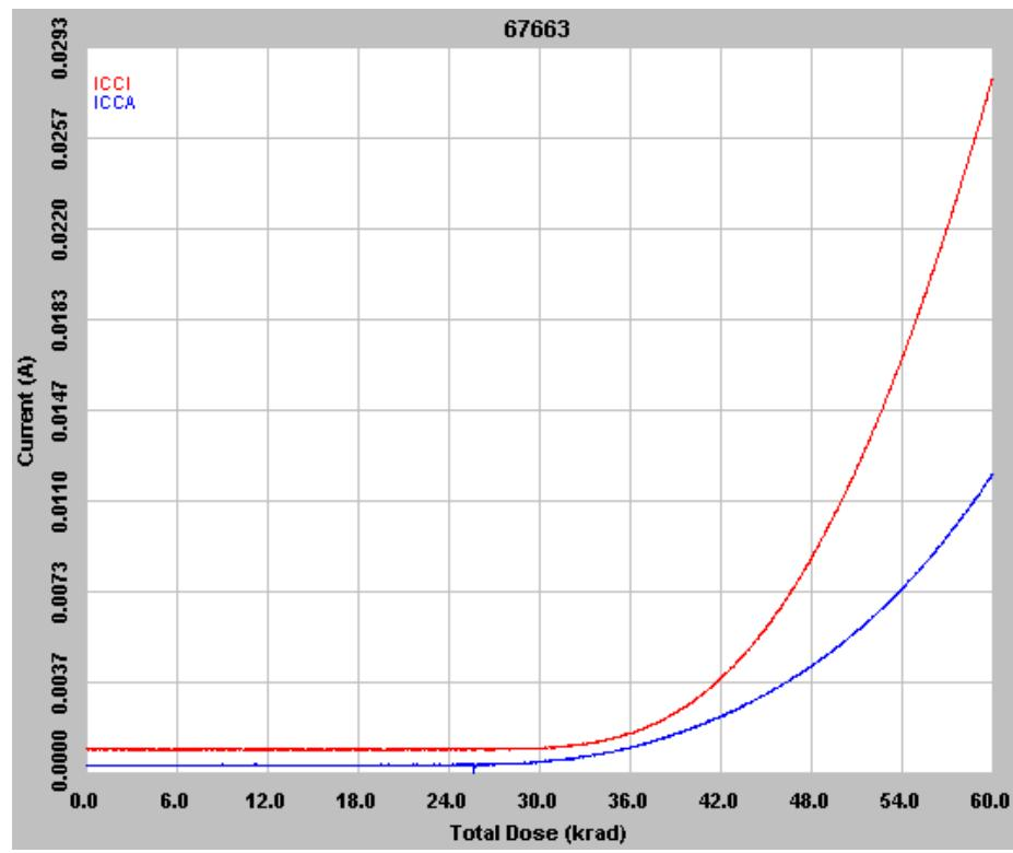
Figure 2 In flux  $I_{CCI}$  and  $I_{CCA}$  of DUT 67663, 60-krad total dose
