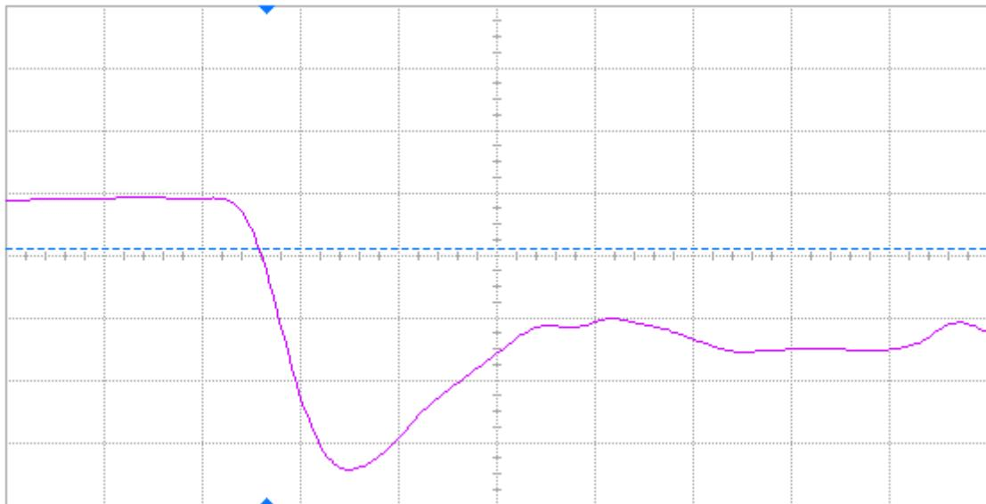
Figure 23 Pre-annealing falling edge of DUT 67771, abscissa scale is 2 V/div and ordinate scale is 2 ns/div.
