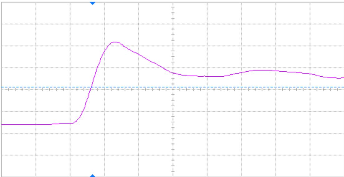
Figure 11 Pre-annealing rising edge of DUT 67741, abscissa scale is 2 V/div and ordinate scale is 2 ns/div.
