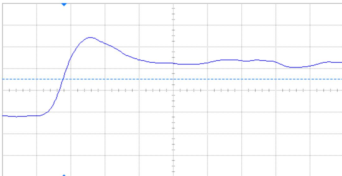
Figure 8 Post-annealing rising edge of DUT 67663, abscissa scale is 2 V/div and ordinate scale is 2 ns/div.
