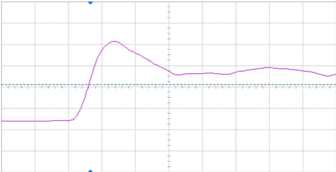
Figure 15 Pre-annealing rising edge of DUT 67774, abscissa scale is 2 V/div and ordinate scale is 2 ns/div.
