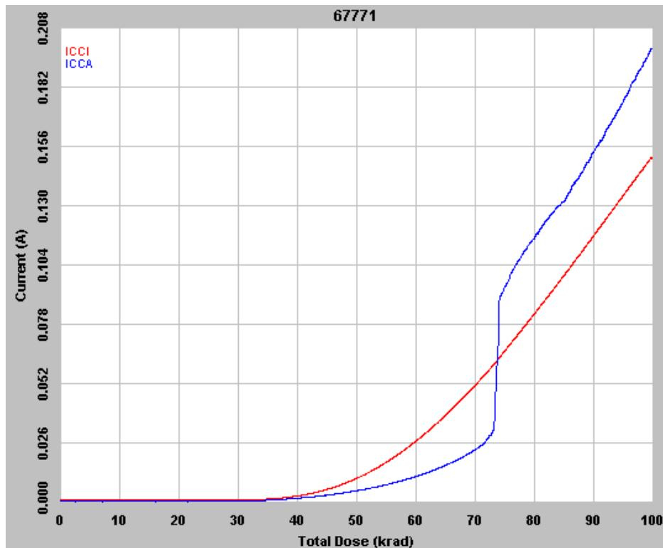
Figure 5 In flux  $I_{CCl}$  and  $I_{CCA}$  of DUT 67771,  $I_{CCA}$  shows a transition near 74 krad that indicates the temporary disabling of the outputs.
