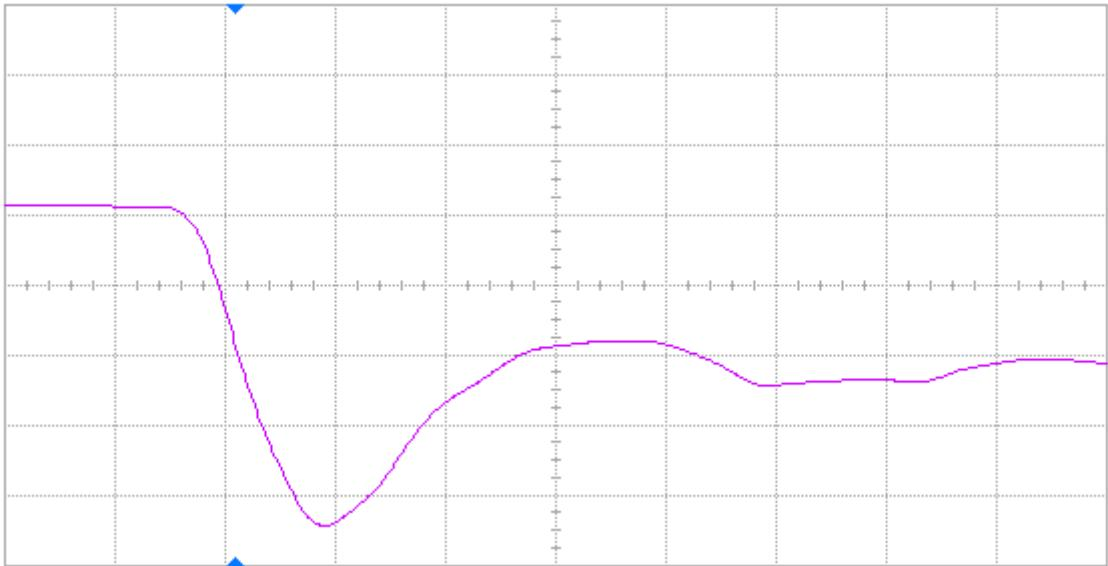
Figure 19 Pre-annealing falling edge of DUT 67714, abscissa scale is 2 V/div and ordinate scale is 2 ns/div.
