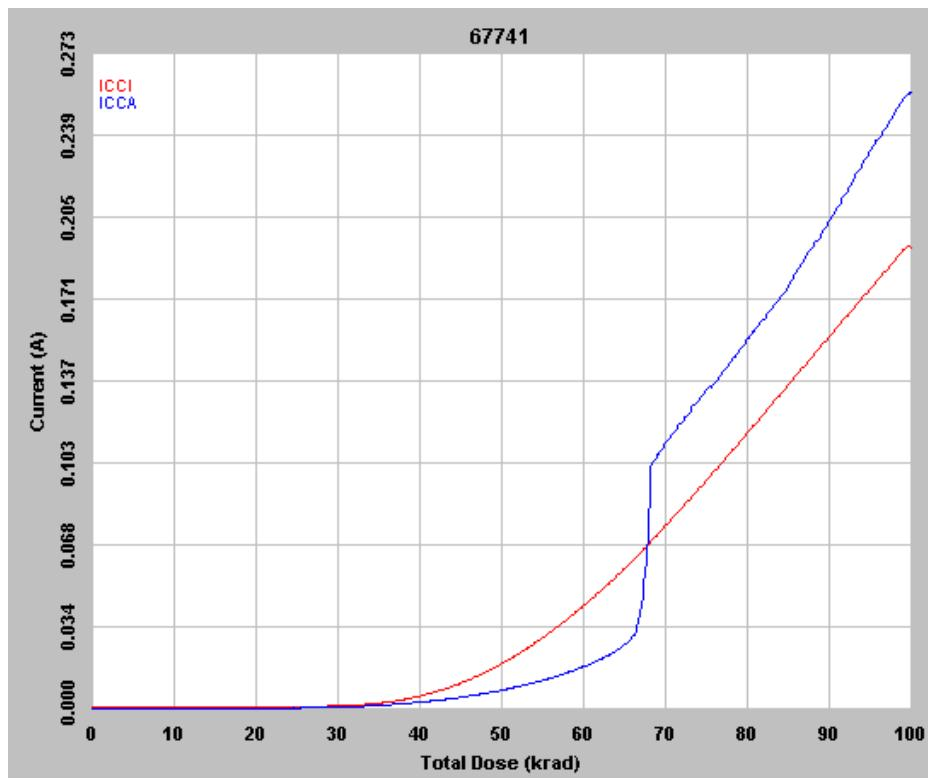
Figure 4 In flux  $I_{CCl}$  and  $I_{CCA}$  of DUT 67741,  $I_{CCA}$  shows a transition near 67 krad that indicates the temporary disabling of the outputs
