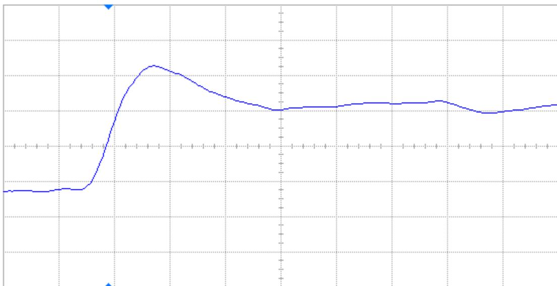
Figure 12 Post-annealing rising edge of DUT 67741, abscissa scale is 2 V/div and ordinate scale is 2 ns/div.
