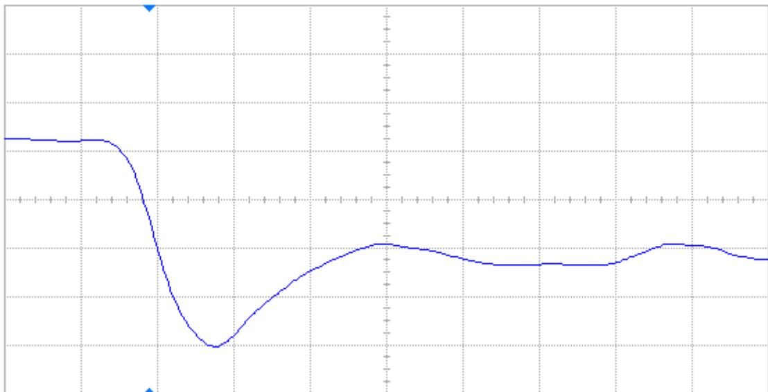
Figure 22 Post-annealing falling edge of DUT 67741, abscissa scale is 2 V/div and ordinate scale is 2 ns/div.
