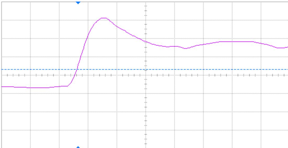
Figure 7 Pre-annealing rising edge of DUT 67663, abscissa scale is 2 V/div and ordinate scale is 2 ns/div.
