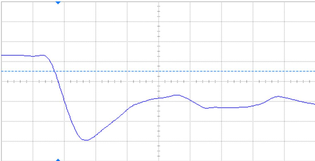
Figure 18 Post-annealing falling edge of DUT 67663, abscissa scale is 2 V/div and ordinate scale is 2 ns/div.
