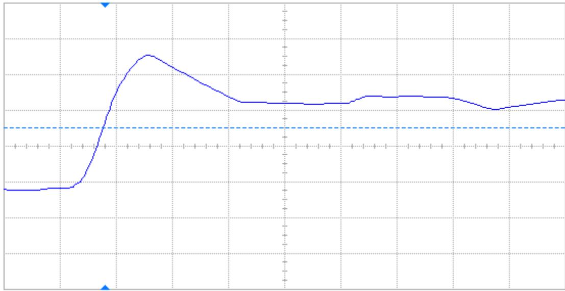
Figure 10 Post-annealing rising edge of DUT 67714, abscissa scale is 2 V/div and ordinate scale is 2 ns/div.
