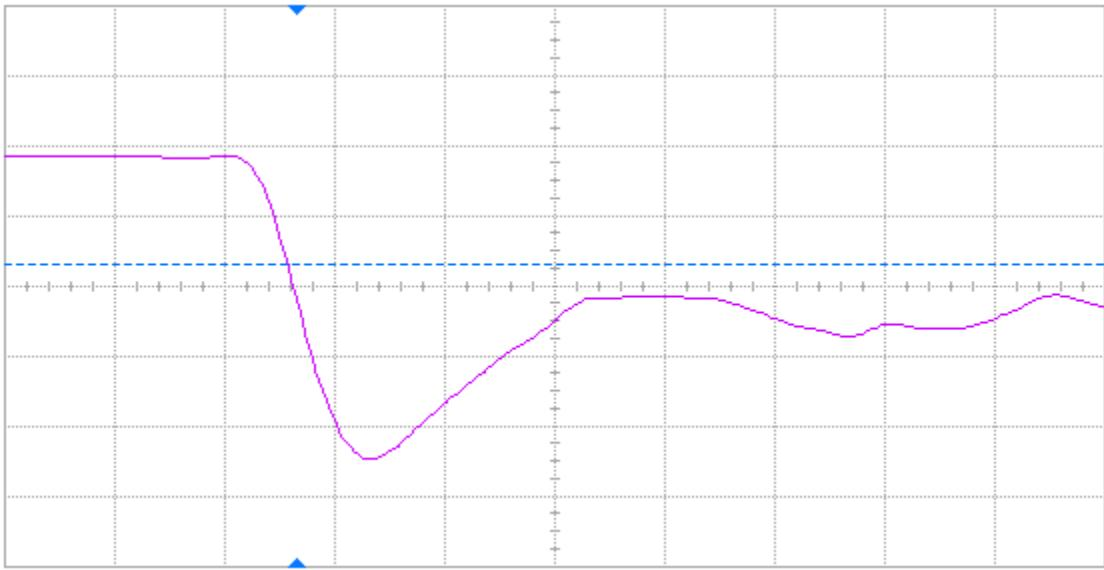
Figure 17 Pre-annealing falling edge of DUT 67663, abscissa scale is 2 V/div and ordinate scale is 2 ns/div.
