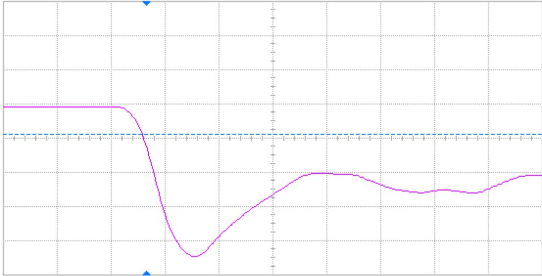
Figure 21 Pre-annealing falling edge of DUT 67741, abscissa scale is 2 V/div and ordinate scale is 2 ns/div.
