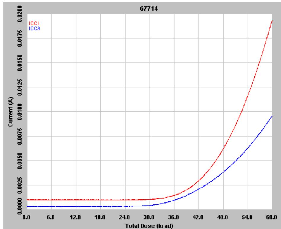
Figure 3 In flux  $I_{CCI}$  and  $I_{CCA}$  of DUT 67714, 60-krad total dose
