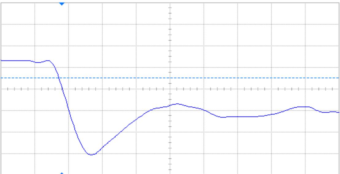
Figure 20 Post-annealing falling edge of DUT 67714, abscissa scale is 2 V/div and ordinate scale is 2 ns/div.
