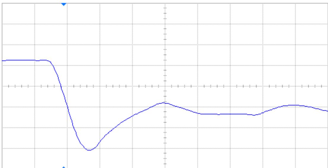
Figure 24 Post-annealing falling edge of DUT 67771, abscissa scale is 2 V/div and ordinate scale is 2 ns/div.
