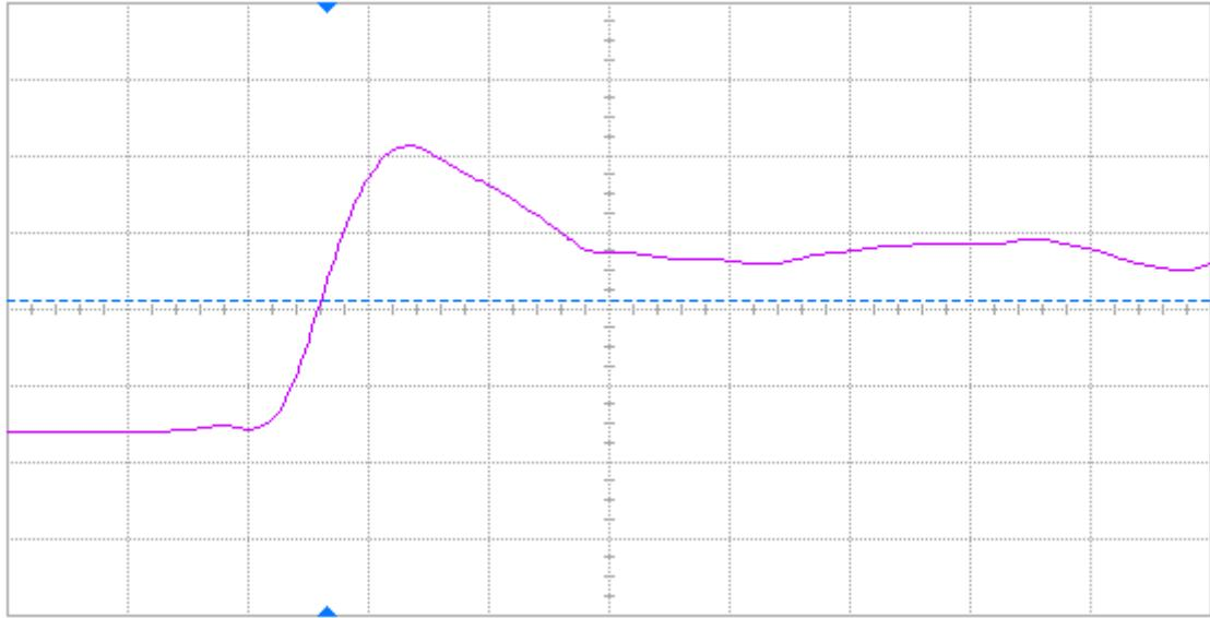
Figure 13 Pre-annealing rising edge of DUT 67771, abscissa scale is 2 V/div and ordinate scale is 2 ns/div.
