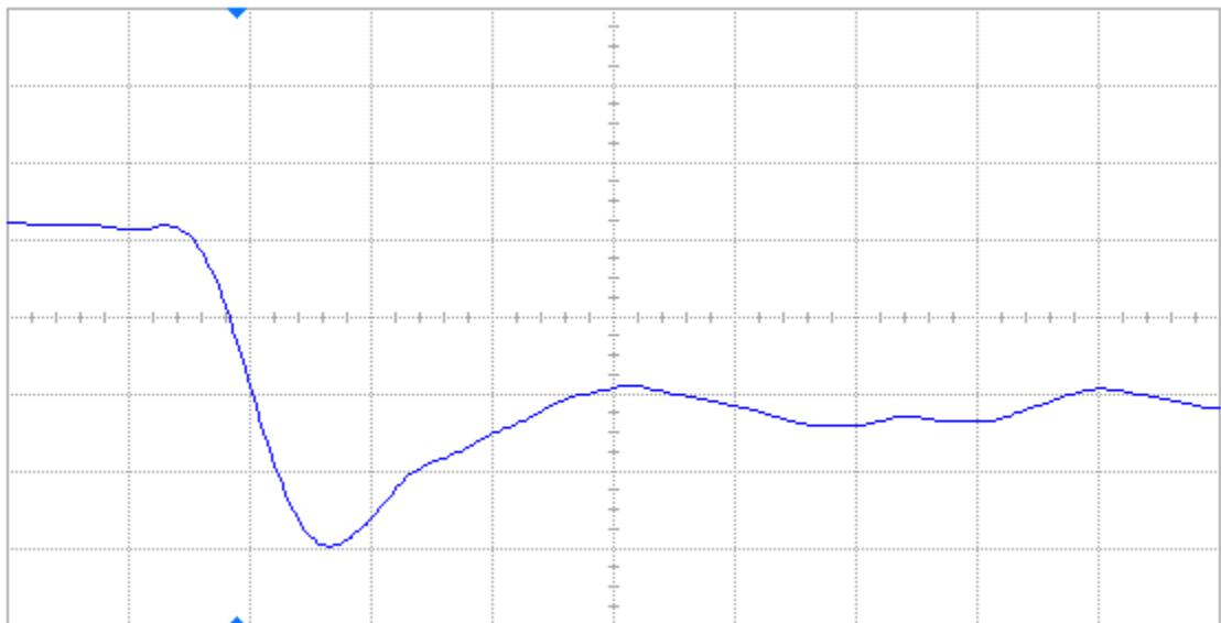
Figure 26 Post-annealing falling edge of DUT 67774, abscissa scale is 2 V/div and ordinate scale is 2 ns/div.
