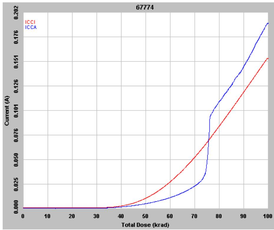
Figure 6 In flux  $I_{CCA}$  and  $I_{CCI}$  of DUT 67774,  $I_{CCA}$  shows a transition near 75 krad that indicates the temporary disabling of the outputs.
