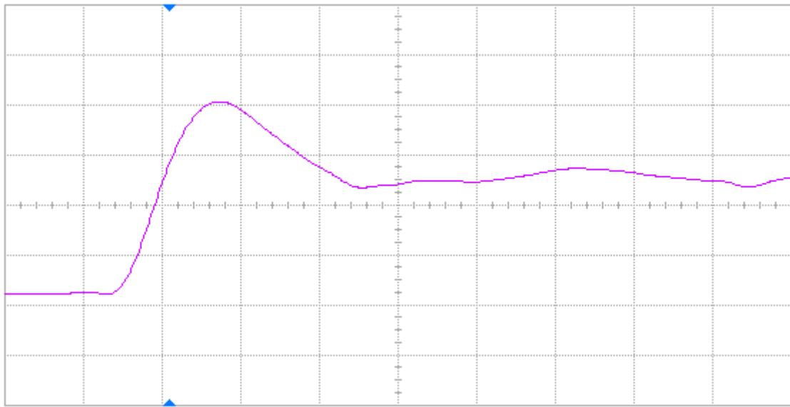
Figure 9 Pre-annealing rising edge of DUT 67714, abscissa scale is 2 V/div and ordinate scale is 2 ns/div.
