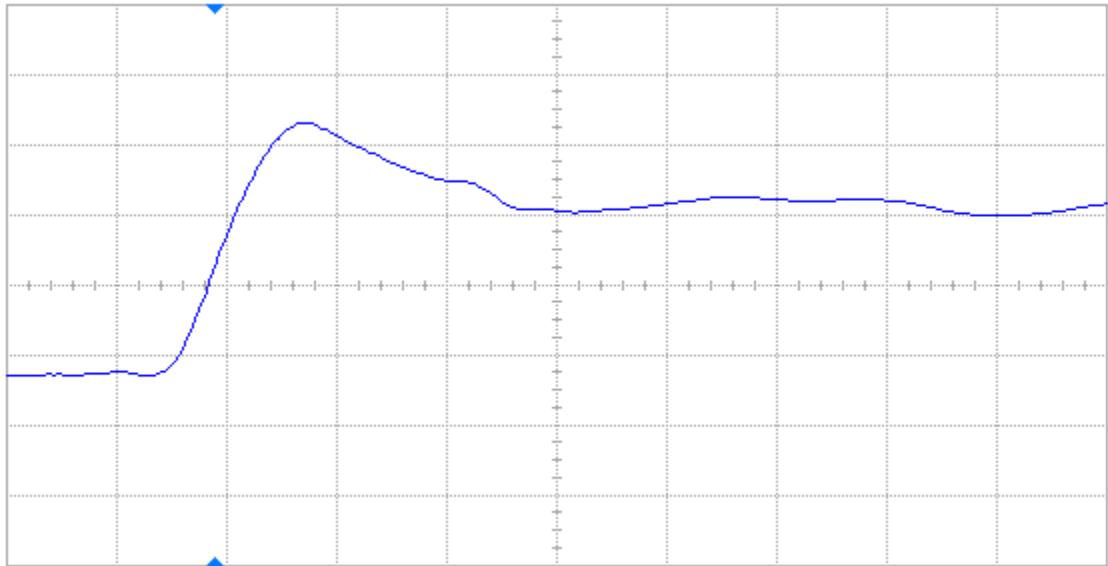
Figure 14 Post-annealing rising edge of DUT 67771, abscissa scale is 2 V/div and ordinate scale is 2 ns/div.
