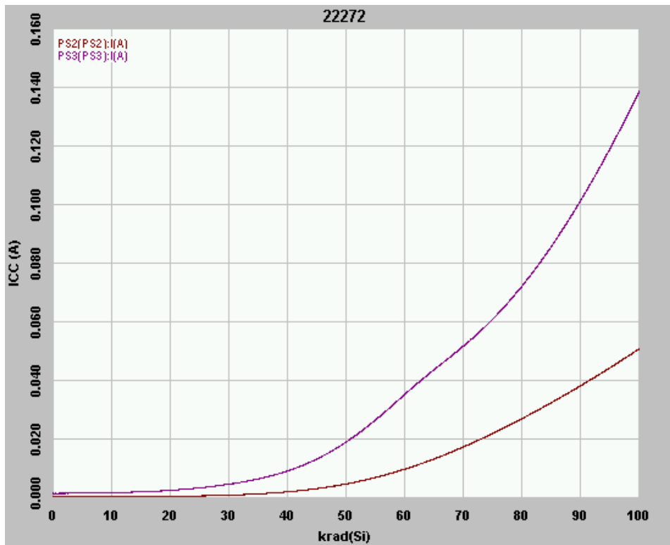
Fig 5 In-flux I_{CC} of DUT 22272, PS2 supplies I_{CCI} and PS3 supplies I_{CCA} .
