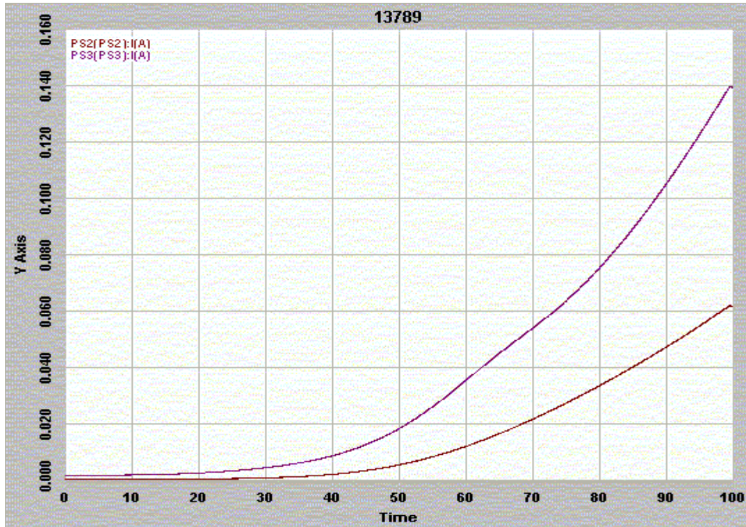
Fig 6 In-flux I_{CC} of DUT 13789, PS2 supplies I_{CCI} and PS3 supplies I_{CCA} . The current unit is amps and the time unit is minutes, 1 minute is equivalent to 1 krad(Si). I_{CC} reaches the peak at 100 krad(Si), irradiation stops after 100 krad(Si) and I_{CC} drops due to annealing effect.
