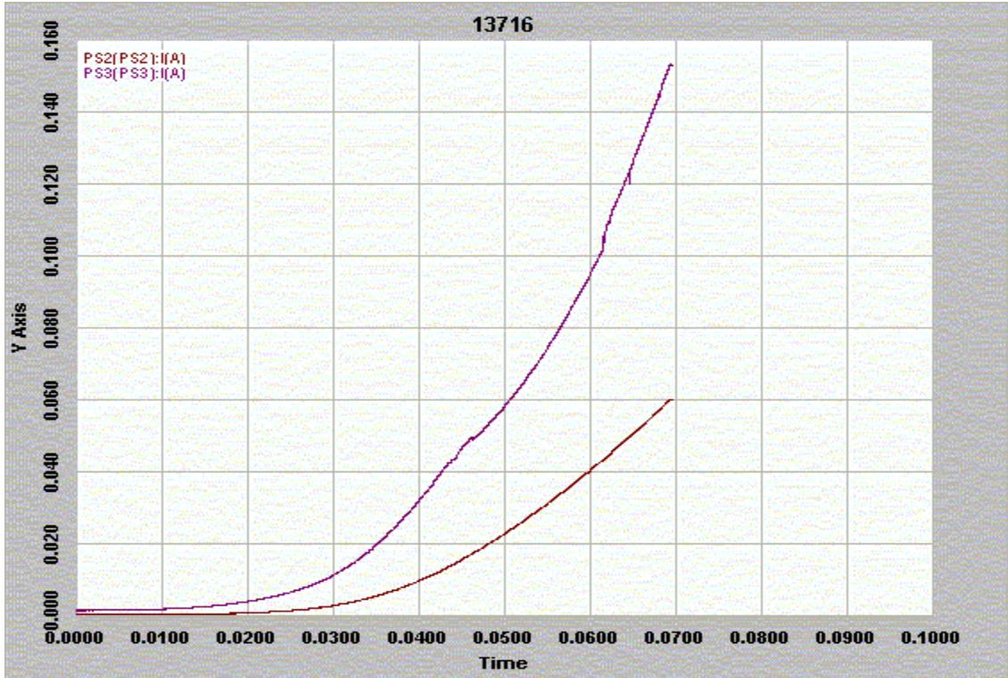
Fig 2 In-flux I_{CC} of DUT 13716, PS2 supplies I_{CC1} and PS3 supplies I_{CC2} . The current unit is amps and the time unit is days, 0.01 day is equivalent to 14.4 krad(Si). I_{CC} reaches the peak at 100 krad(Si), irradiation stops after 100 krad(Si) and I_{CC} drops due to annealing effect.
