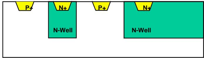
**FIGURE 2: Super-Guardring in High Voltage**
