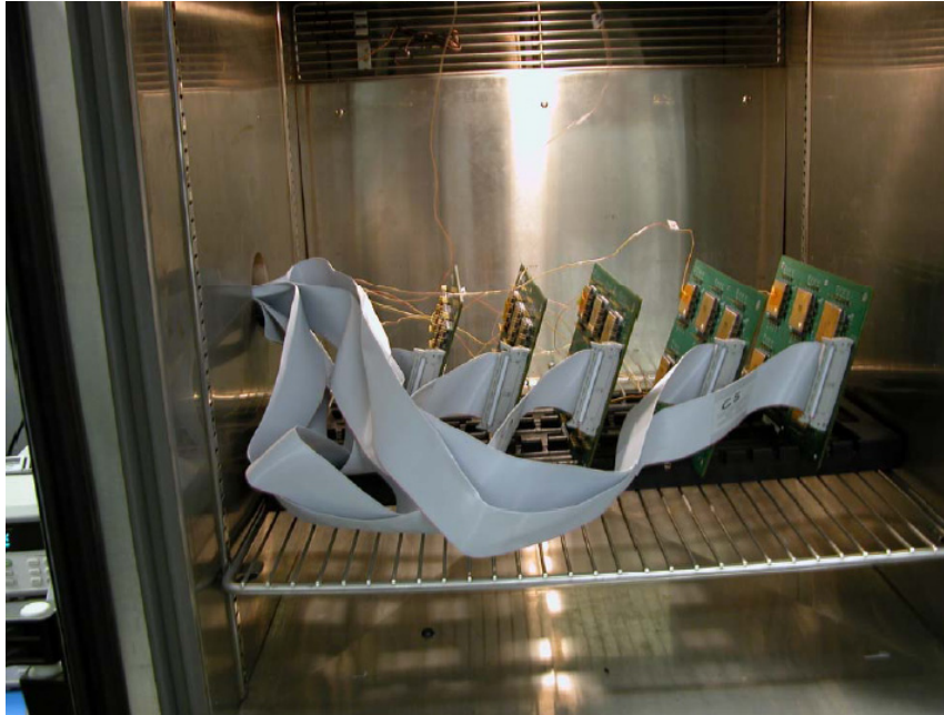
Figure 5: Testing PCB's in Oven
