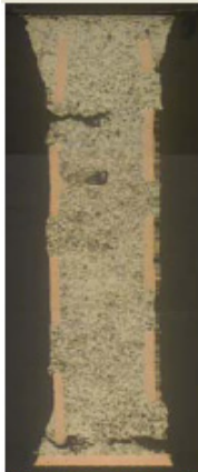
CG1152 80 Pb / 20 Sn, Cycle 1225 1 st failure at cycle 1212
