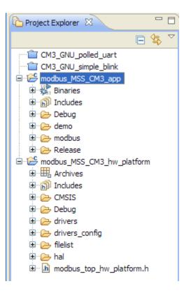
Note that the first two projects are closed while the other two projects are the application and library projects generated by Libero from the associated hardware project. Many commonly used project operations can be carried out by left mouse button clicking on a project in the **Project Explorer** to select it and then choosing the appropriate menu option or toolbar button, or by right mouse button clicking on the project and choosing an option from the context menu that appears:
