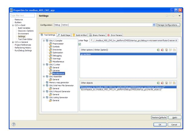
Very often the CMSIS/HAL example linker scripts can be used either as-is or having been adapted to match the needs of a specific target system.
