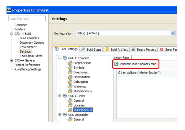
The linker map file created during your build is used to produce information about where symbols are mapped by the linker (including whether a symbol was actually defined by the linker rather than by any particular input file). The linker map also describes allocation of storage in the resulting binary.
