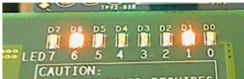
Figure A-1 • Display with LED1 and LED6 ON
