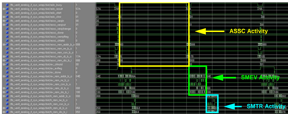
Figure 11-7 • Simulation Result Illustrating Soft IP Events
