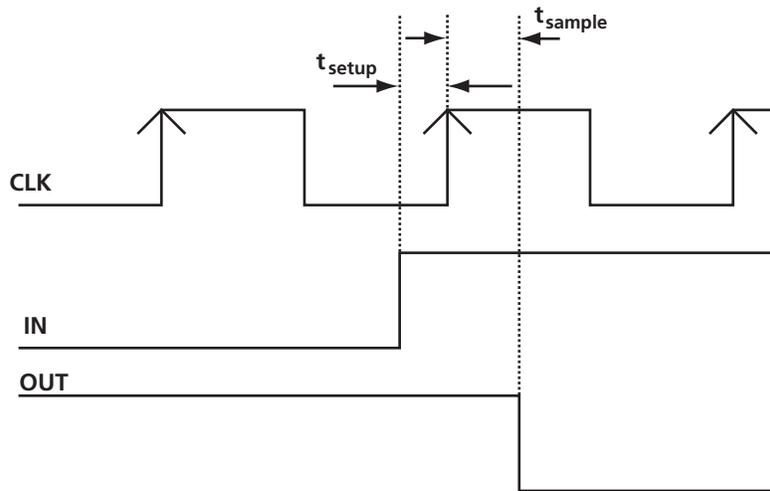
Figure 3 • Timing for the Sample Logic Circuit
