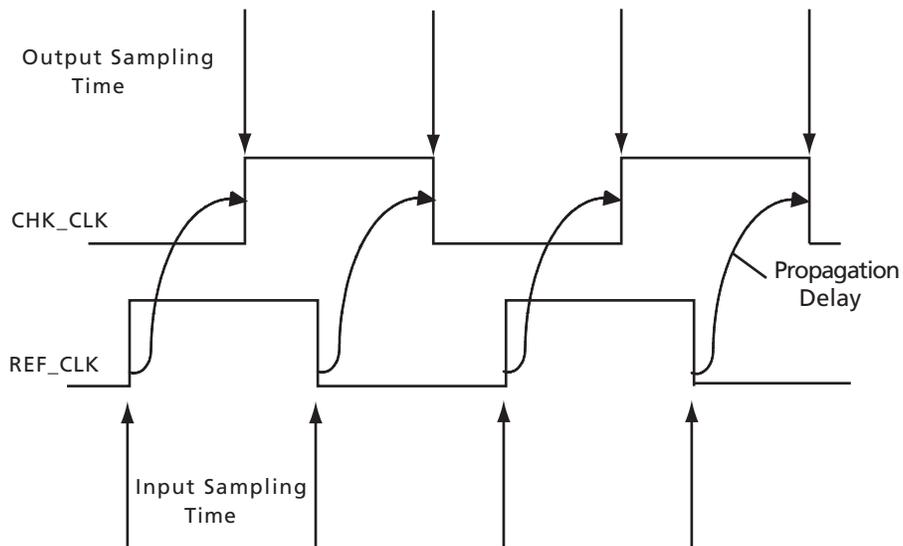
Figure 4 • Input and Output Sampling Time With Respect to the Reference Clock and Virtual Clock
