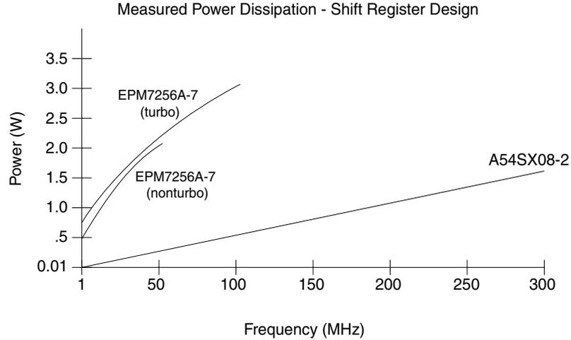
**Figure 1 • Power Requirements - Shift-Register Design**
