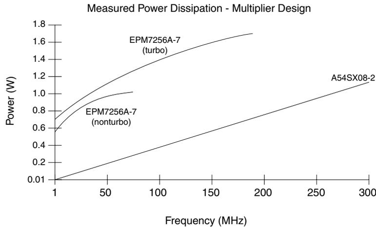
**Figure 2 • Power Requirements - Multiplier Design**
