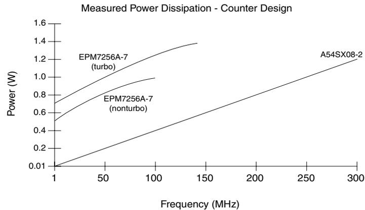
**Figure 3 • Power Requirements - Counter Design**
