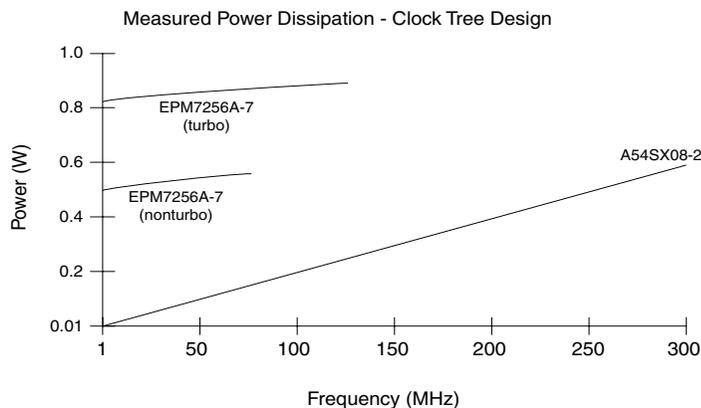
**Figure 4 • Power Requirements - Clock-Tree Design**
