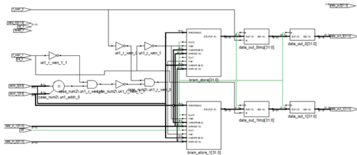
The FPGA synthesis tool infers SmartFusion2 RAM1K18.
