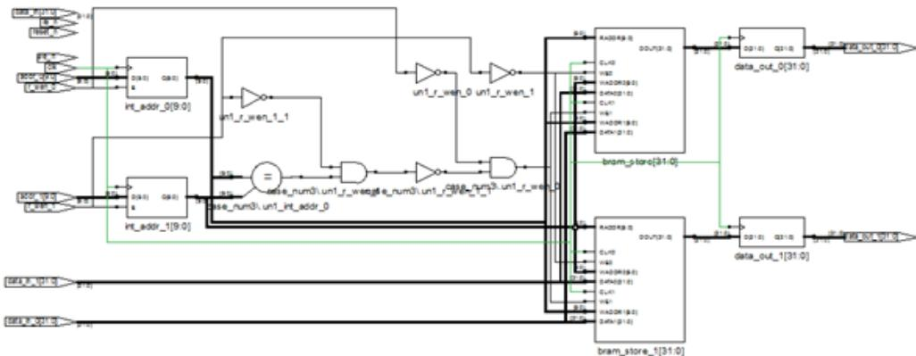
The FPGA synthesis tool infers SmartFusion2 RAM1K18.
