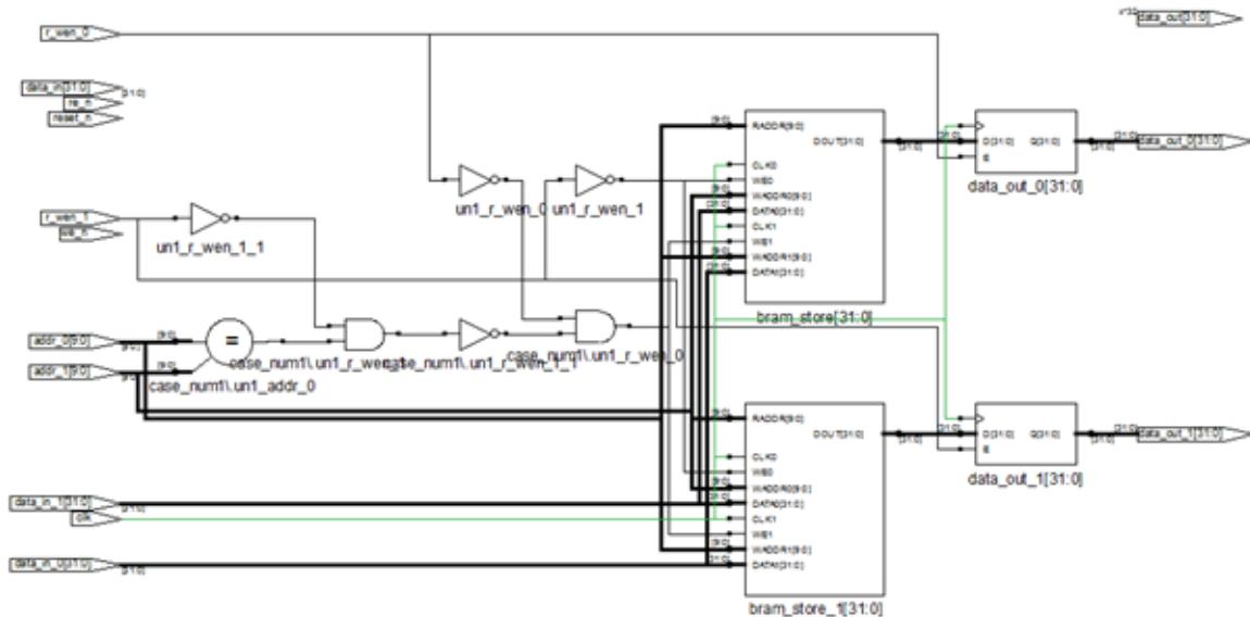
The FPGA synthesis tool infers SmartFusion2 RAM1K18.
