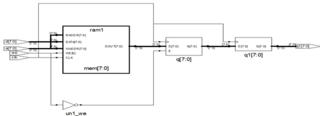
The pipelined register q1 [7:0] optionally can have asynchronous/synchronous reset or clock enable. The software does not pack pipelined register q1 [7:0] if the register q [7:0] has an asynchronous/synchronous reset.
