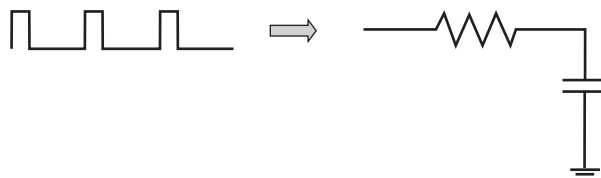
Figure 3 • Converting a PWM Output into a DC Level
