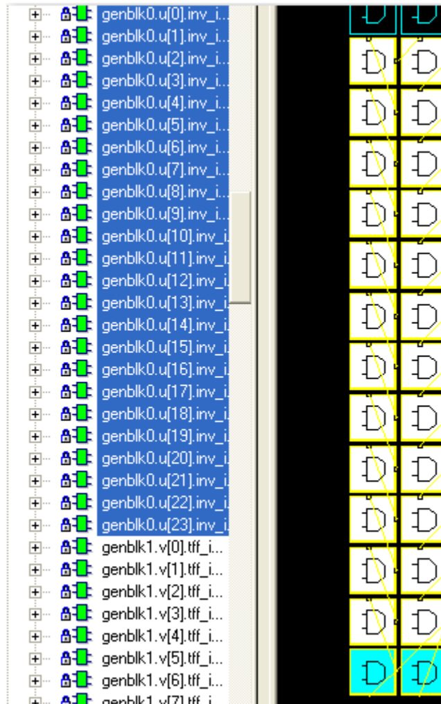
Figure 2 • Ring Oscillator Inverter Loop Placement
