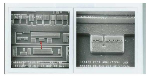
Figure 3 • SEM Photograph of Damaged N3b Transistor
