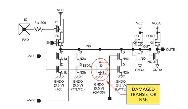
Figure 2 • User I/O Circuit Schematic
