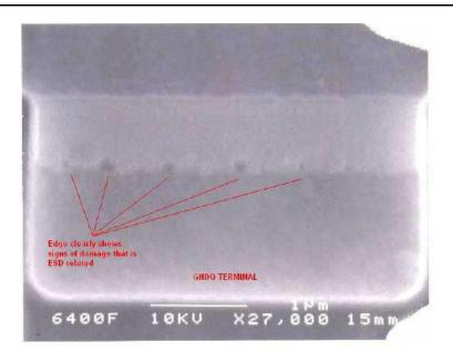
Figure 4 • SEM Photograph of Subtle Damage to N3b Transistor
