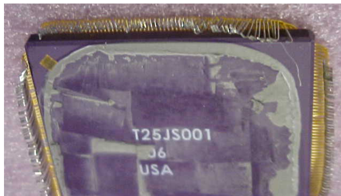
Figure 1 • Improperly Extracted Device
