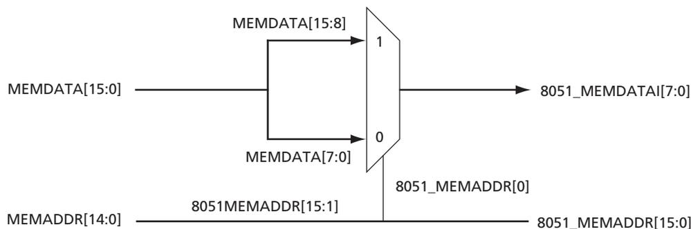
Figure 5 • Byte Read Implementation for Core8051
