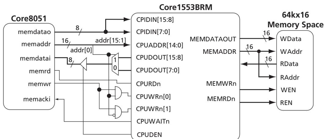
Figure 6 • Using Core1553BRM CPU Interface with Core8051
