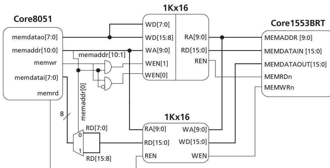
Figure 3 • Design Example with Direct Access to Memory
