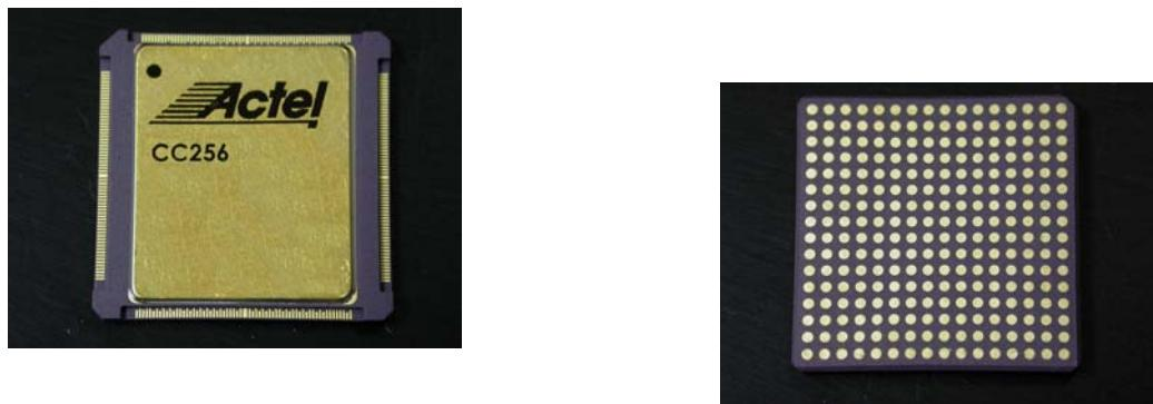
Figure 2 • CC256 Package Top and Bottom View
