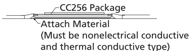
Figure 5 • CC256 Attach Material Drawing
