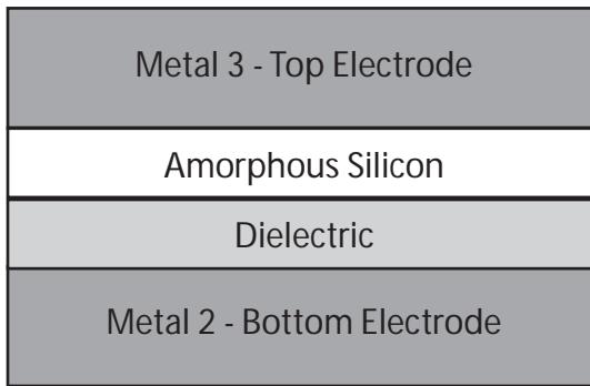
Figure 1 • Cross-sectional View of a Metal-to-Metal Antifuse
