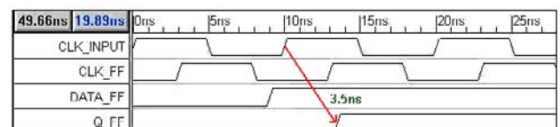
Figure 5 • Example of a Timing Diagram with Large Clock-to-Out Performance
