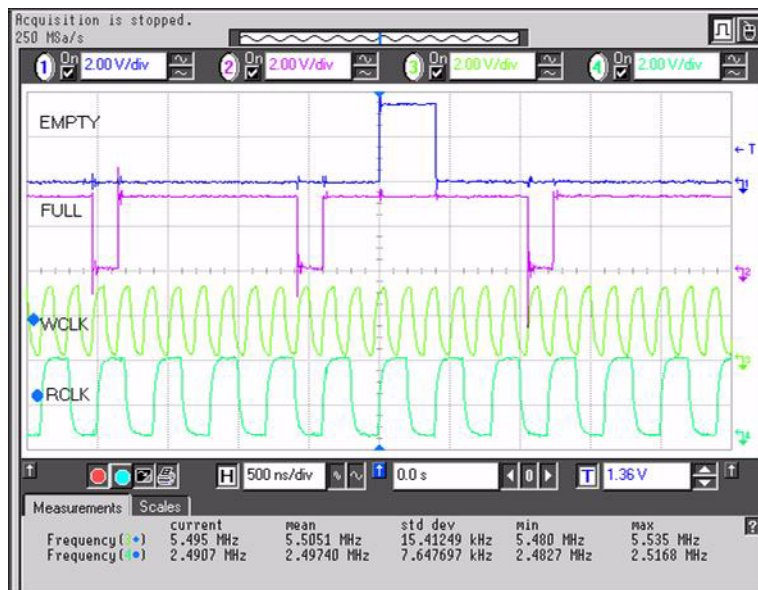
Figure 15 • EMPTY Flag Behavior When RCLK and WCLK Are Not in Phase
