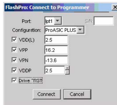
Figure 3 • Drive TRST to '1' from FlashPro or FlashPro Lite
