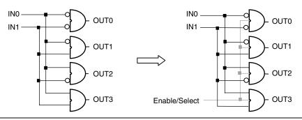
Figure 19 • Decoder with Enable
