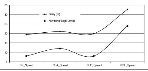
$\textbf{\textit{Figure 6}} \quad \bullet \quad \textit{Number of Logic Levels for various 32-bits Adder Architectures}$
