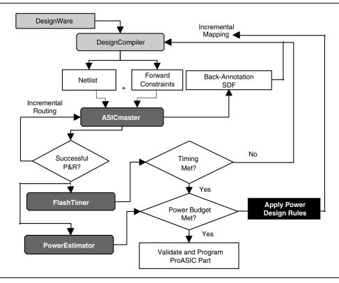
Figure 21 • Block Diagram Design Methodology
