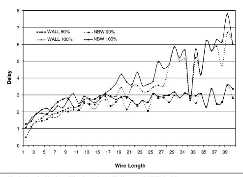
$\textbf{\textit{Figure 9}} \quad \bullet \quad \textit{Delay Variation for Various Wire Lengths in Wallace and NBW Architectures}$
