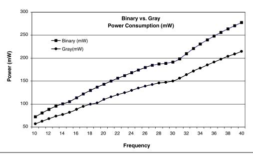
Figure 10 • Comparative Power Consumption for 200 instances of 8-bit Counters
