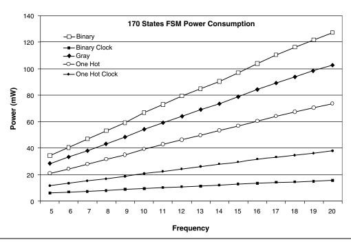
Figure 11 • Power Measure on ProASIC of 170 States Controller
