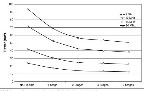
Figure 13 • ProASIC Power Characterization for 16-Bit Pipelined Multipliers
