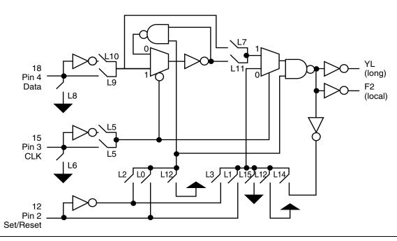
Figure 2 • Architecture of the Logic Tile
