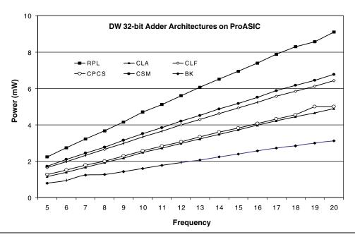
Figure 4 • ProASIC Silicon Power Characterization for Various 32-bit Adders
