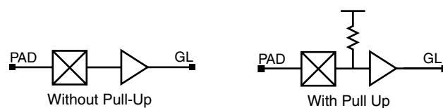
Figure 2 • 3.3V/2.5V Global Input Pad Cells
