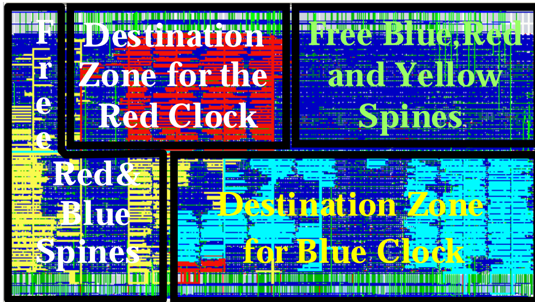
Figure 5 • Limitation of the Clock Scope and Economy of Low-Skew Spines
